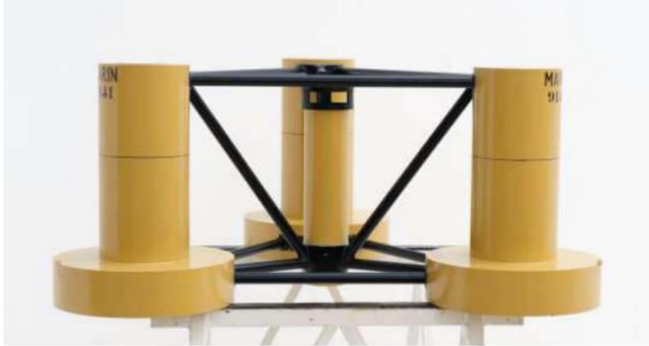
Figure 4.2 – As-built picture of DeepCwind semisubmersible for 1/50th scale tests (OC4) (NREL/TR-500-38060)
