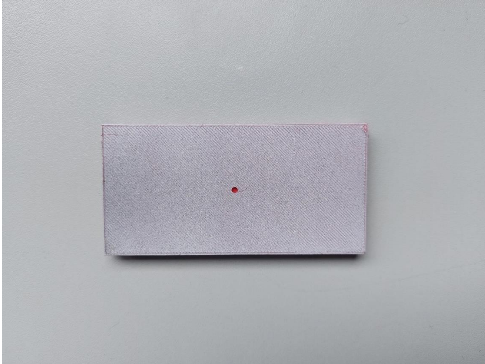
Figure 23 - Drilled specimen used for the DIC strain measurement approach.
