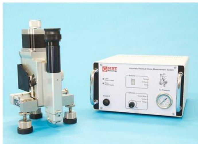
Figure 18 - Automatic system for the measurement of residual stresses, MTS3000-Restan (SINT Technology, 2021).
