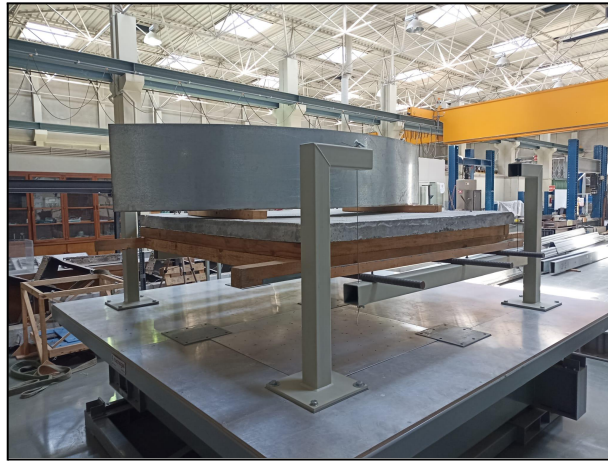
Figure 3.2 - Big scale model with the quarter-ring TLD fixed to the shaking table.
