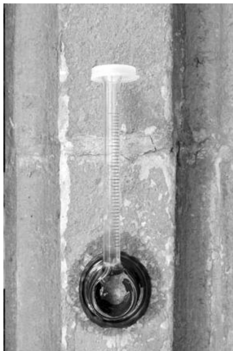
Figura 18 – Tubos de Karsten in situ [27].
