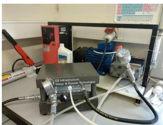
Figure 5.1 – Experimental set-up used in ultra and nanofiltrations.
