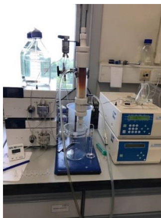
Figure 5.2 - Chromatographic installation used in the adsorption/desorption experiments.
