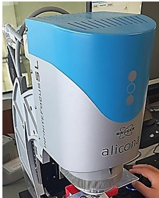
Figure 36. Measurement of internal hole surface roughness using the ALICONA Infinite Focus SL.
