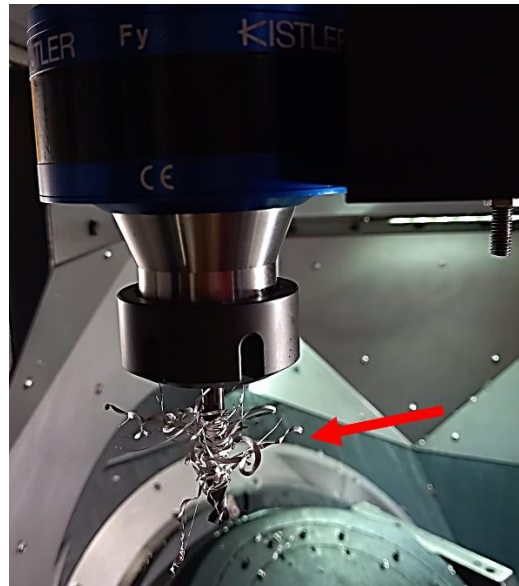
Figure 58. Chip adherence to the drilling tool 2 observed during the drilling campaign (ii).
