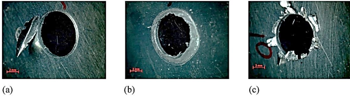
Figure 18. Distinct types of burr formation: (a) uniform with drill cap; (b) uniform without drill cap; (c) crown-shaped burr [68].
