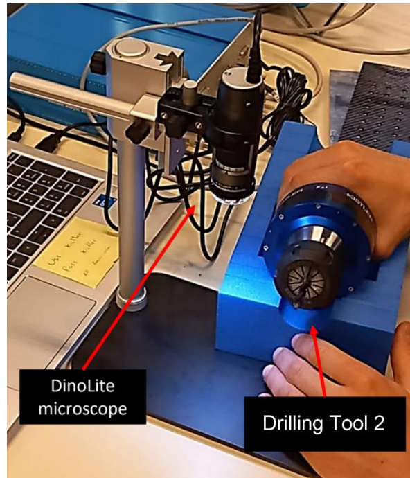
Figure 37. Images of wear analysis in the drilling tool 2 taken in the DinoLite digital USB microscope.
