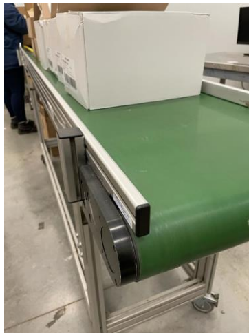
Figure 13 - Conveyor side bars.
