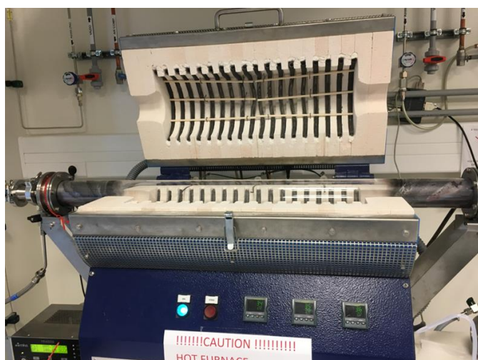
Figure 3-2 - Tube furnace used for the annealing treatment.
