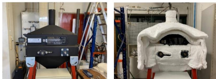
Figure 2: Experimental installation (without and with thermal insulation).
