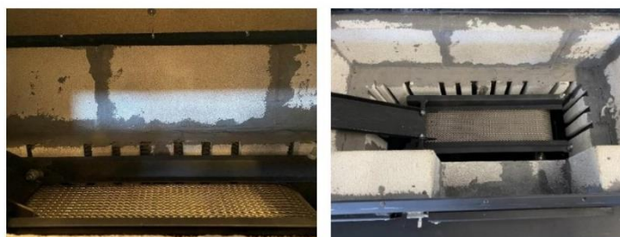
Figure 3: Traveling grate (front view and top view).
