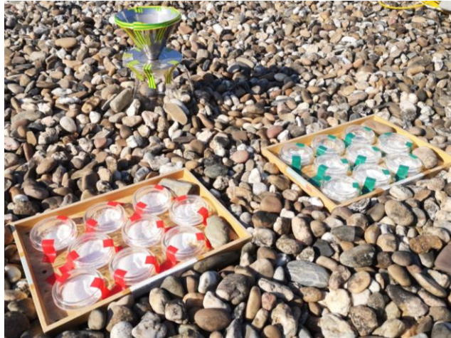
Fig. 3.5. Rooftop weathering experimental setup: rainwater filtration and collection system (above) and perforated trays with microplastic particles in Petri dishes (below).
