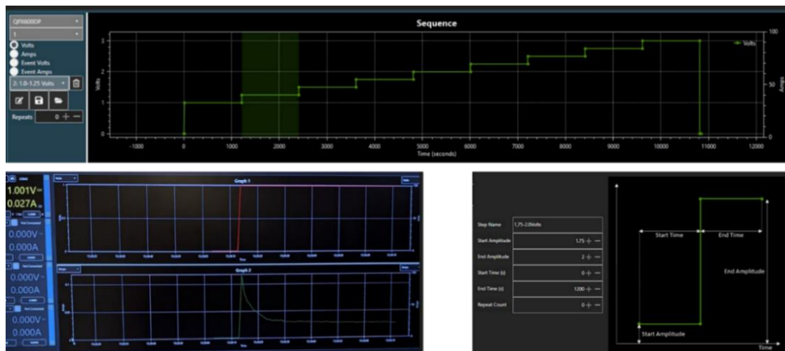
Figure 19 - Chronoamperometry step test sequence (on the Top) below it is represented the sequence modelling parameters (on the right side) and the programme Test bridge plots to analyse the voltage and current evolution during the experiments (left).
