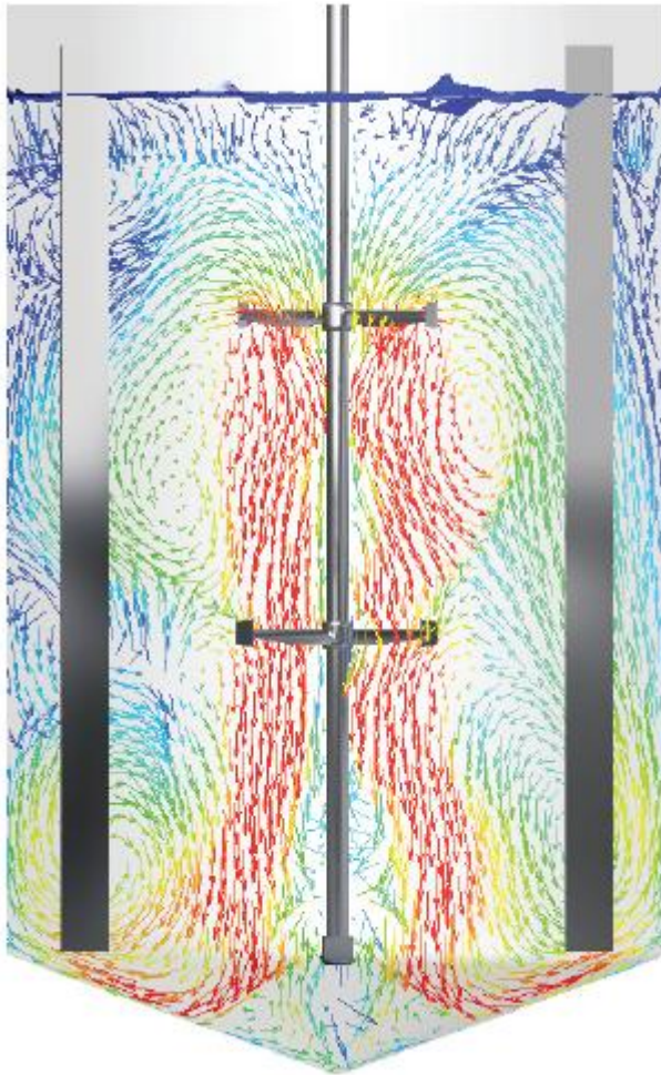
Figure A.2.3 - This simulation is indicative at the viscosity level and may not coincide with the viscosity of the product in the quotation.
