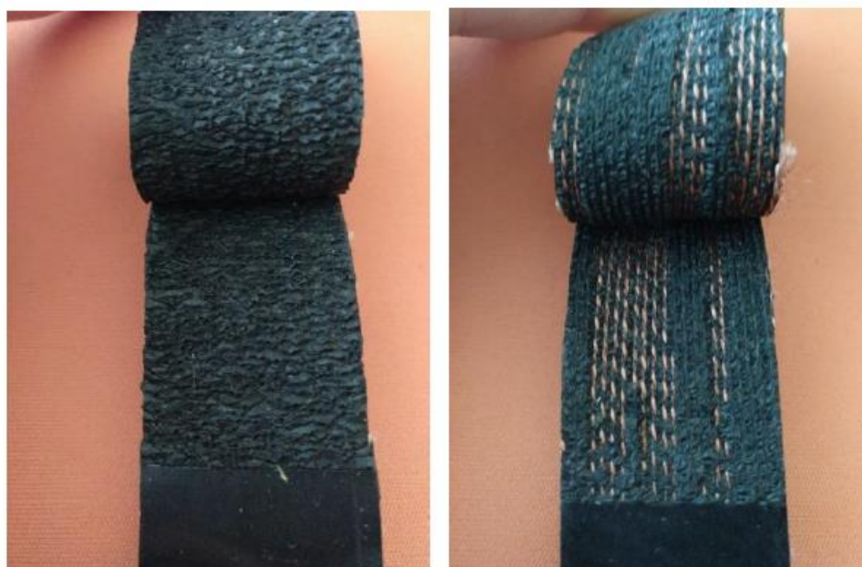
Figure B.1 - Example of a peel adhesion test results: showing a good result, on the left, and a bad one on the right (Rocha, 2019).
