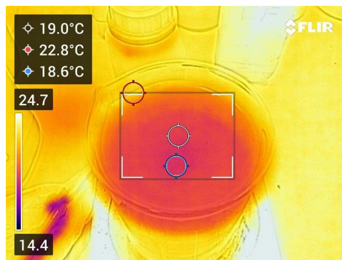
Figure B.1.6 - Dipping solution temperature for T = 19.0\text{ }^{\circ}\text{C} trial.
