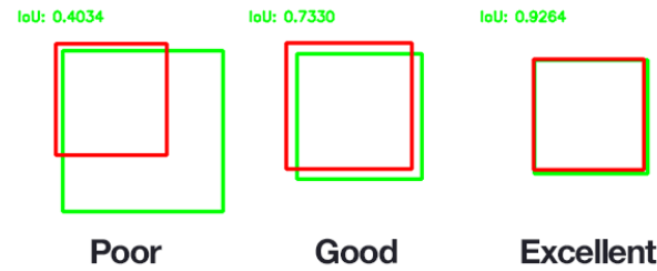
Figure 2.5: Demonstration of the IoU metric. Green rectangle is the ground-truth and the red one is the predicted. [3]
