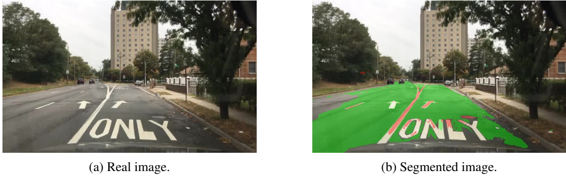
Figure 6.8: Demonstration of the HybridNets segmentation on real dataset.
