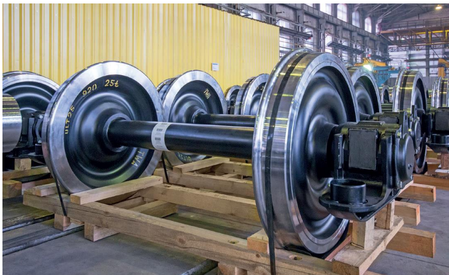
Figure 2-1 - Modern wheelsets manufactured by K LW WheelCo. Taken from K LW WheelCo SA (2019)
