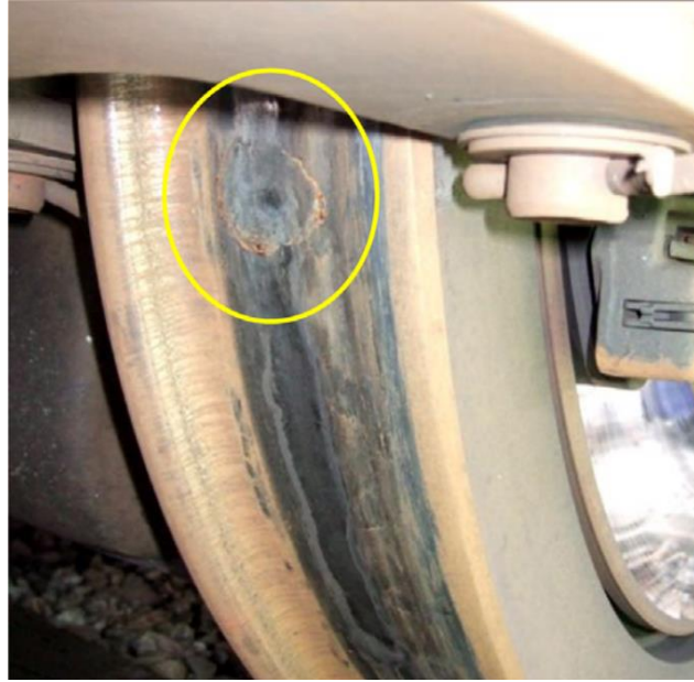
Figure 2-4 - Wheel flat formed by wheel–rail slip in the contact. Taken from Steenbergen (2008)
