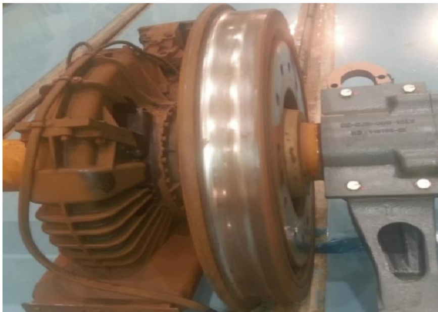
Figure 2-9 - Defected wheel with polygonization. Taken from Jin et al. (2018)
