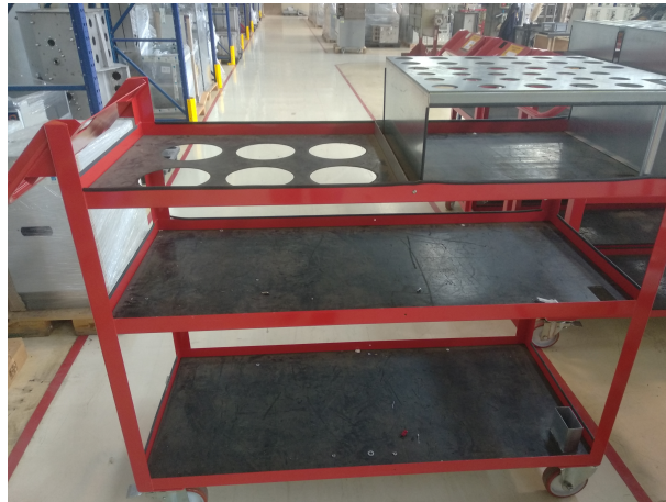
Figure 3.20: Fluofix picking cart
