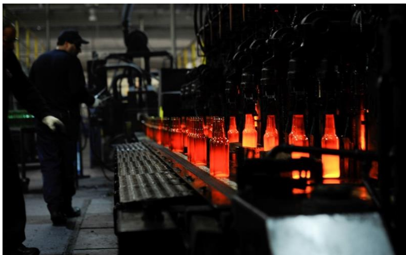
Figure 3.1: Bootles after final moulding (Larguesa 2015)
