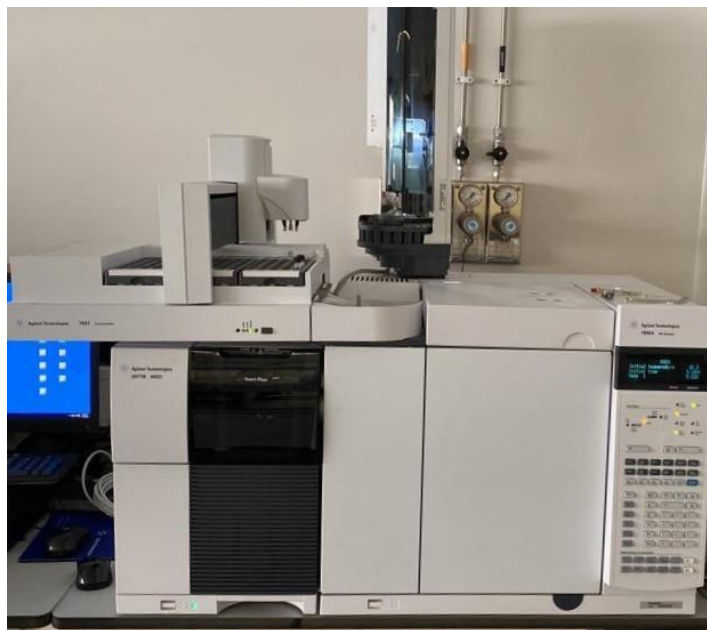
Figure 5. Gas chromatograph with mass spectrometry from Agilent Technologies used in the assays.
