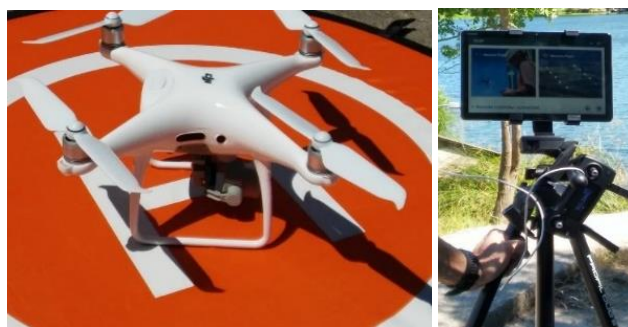
Figure 3.4 – Hardware used for the field data collection. From left to right, “Phantom 3 pro DJI” UAV used for the collection of high-resolution images; tripod with hardware for the automatic flight route of the UAV.
