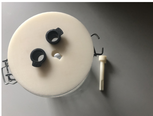
FIGURE 4.9: Electrochemical cell and sample holder drawn for electrochemical experiments using as print material ABS P340.
