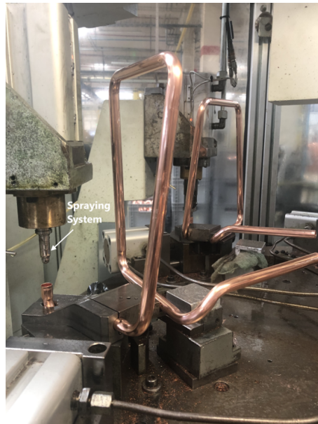
FIGURE 3.5: Cold water coil: flare formation.
