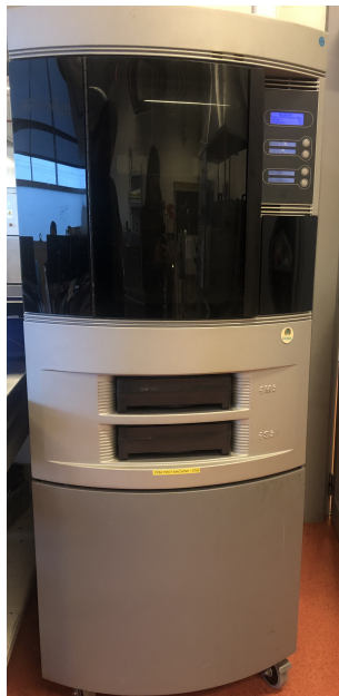
FIGURE D.2: The 3D printer Stratasys dimension elite used to design the morphology of the electrochemical cell, whose operations is based on FDM (Fused Deposition Modeling) technology. The impression material used was ABS P340 amorphous polymer (Stratasys).
