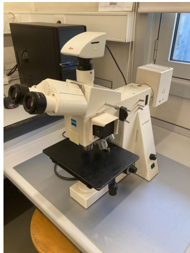
FIGURE 4.6: Optical Microscope ZEISS Axiotech used to record different microstructures of copper samples.
