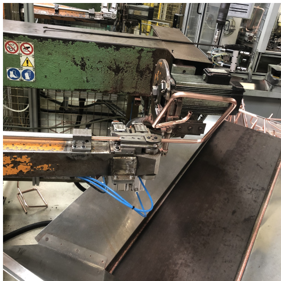
FIGURE 3.4: Machine used for coils manufacturing.
