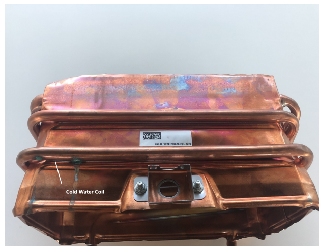
FIGURE 1.1: Illustration of the coil of the heat exchanger where 78% of the failures occur.
