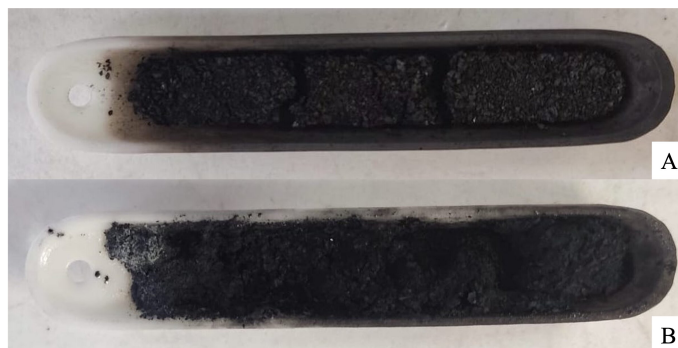
FIGURE 3.9: Ceramic boat with carbonised PS (A) and with activated PS (B).
