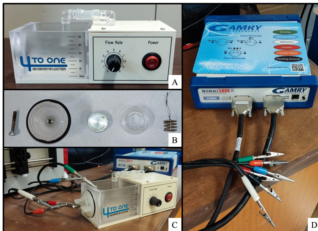
FIGURE 3.12: Experimental apparatus which includes the testing kit (A), the parts to join the anode and the cathode compartments (B) and the potentiostat (D), being all connected like it is seen in (C).
