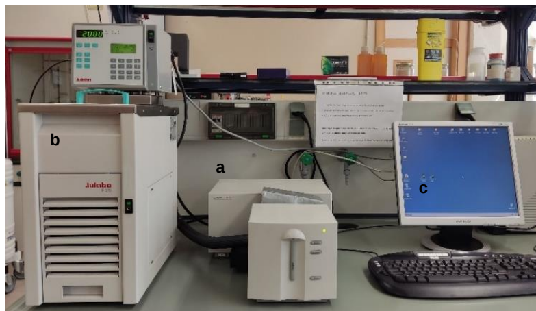
Fig. 20: Setup of the Agilent 8453 UV-Vis Spectrophotometer (a). The apparatus is adjoined to a circulating water bath (b) which keeps the cell holder at a fixed designated temperature. The device is also connected to a pc interface (c) for data acquisition.
