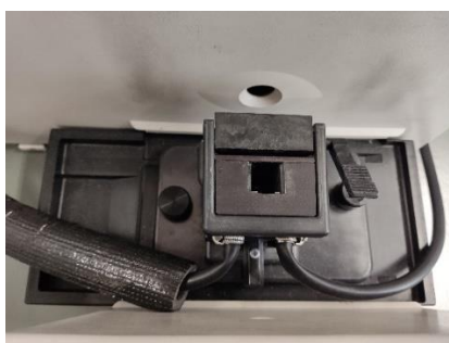
Fig. 21: Temperature control of the cell holder via a circulating water bath.
