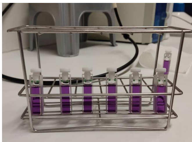
Fig. 39: Optical glass cells with solutions of C_{60} and different anthracene initial concentrations prepared for the equilibrium study in the reactor.
