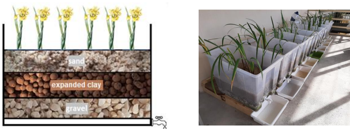
Figure 1 – Schematic representation of the composition of the constructed wetland units and lab scale vertical flow constructed wetland.
