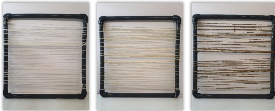
Figure 10- Indoor trial with different types of ropes (cotton, linen, and hemp).
