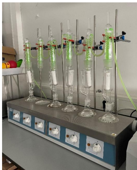
Figure 14: Fat extraction by Soxhlet method.
