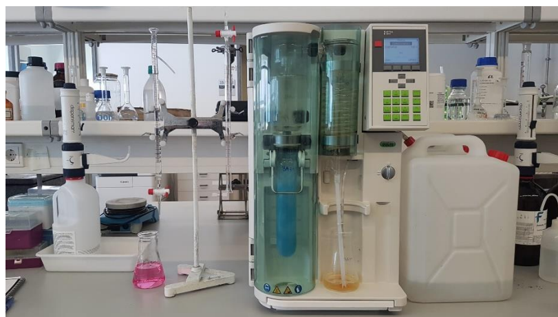
Figure 16: Kjeldahl Distillation Unit and titration.
