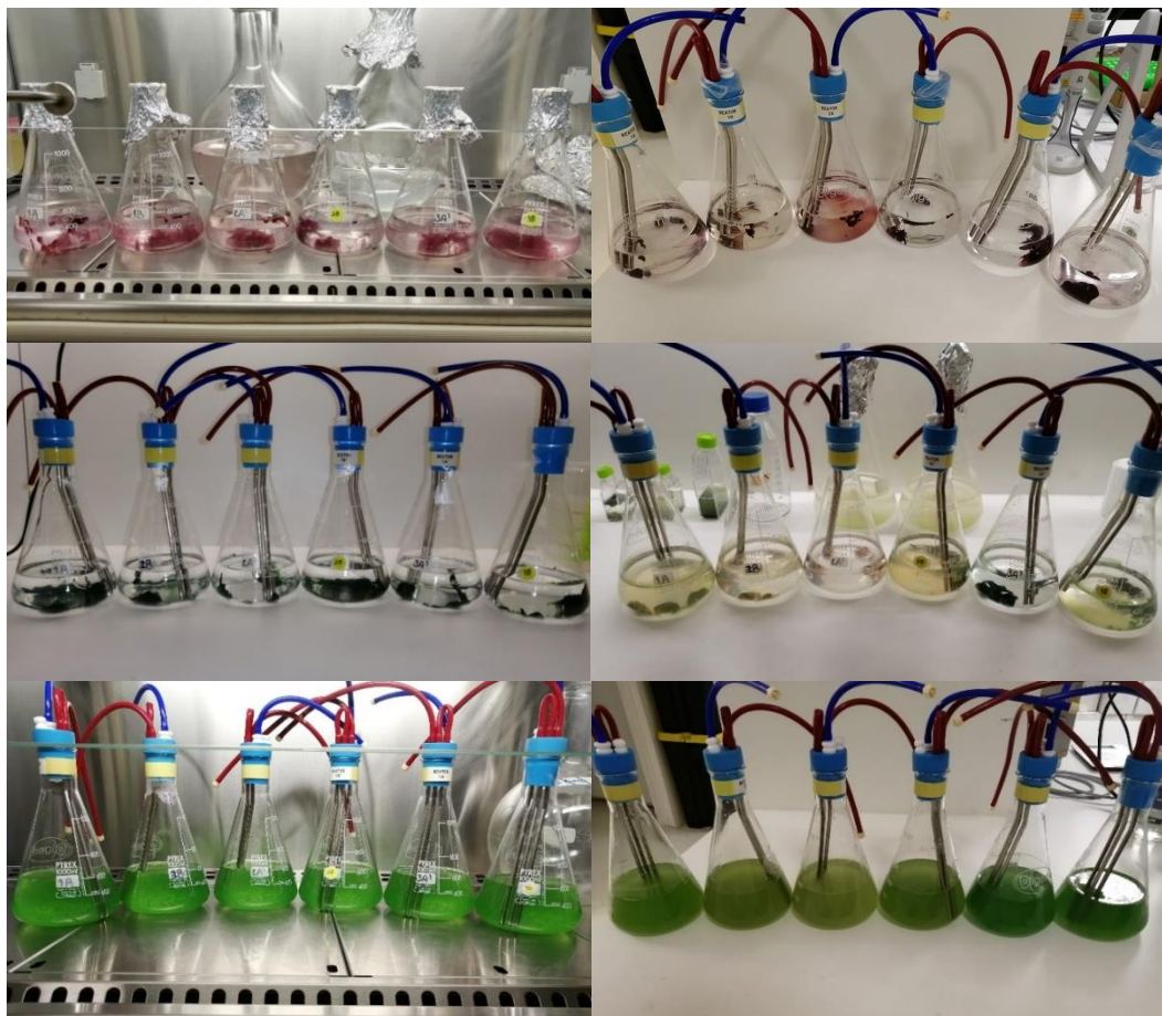
Figure V.1 – Images showing the Algem® Erlenmeyer flasks containing the cyanobacterial strains before (left) and after (right) the three-week assay under different light conditions (Top – Spirulina sp. LEGE 11439; Middle – Spirulina sp; Bottom – Arthrospira platensis PCC 7345).
