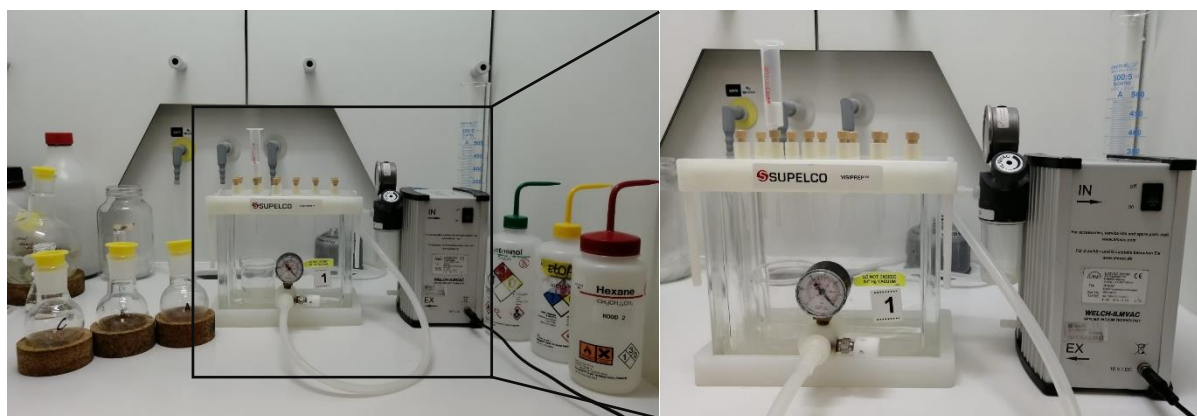
Figure IV.2 - Instrument setup used in the fractionation of each extract from the three cyanobacterial strains.
