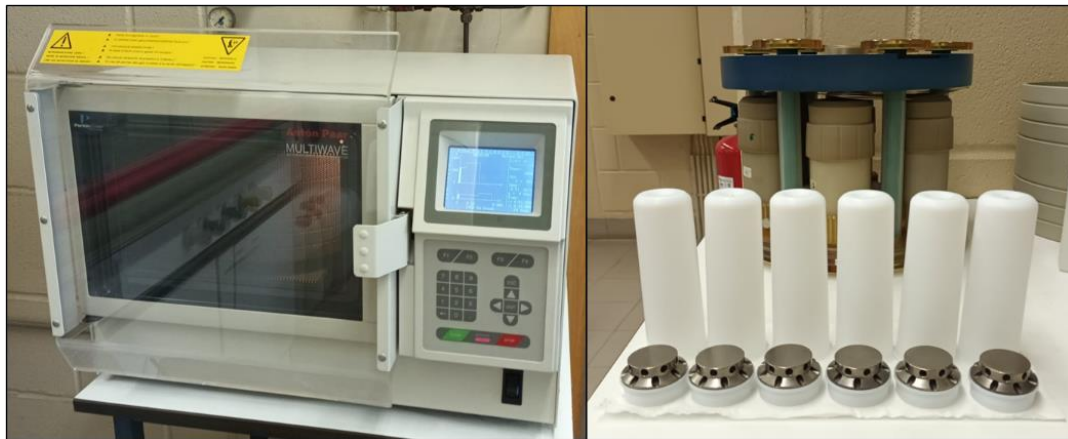
Figure 9 - Microwave-assisted digestion system consisting of oven, rotor and vessels.
