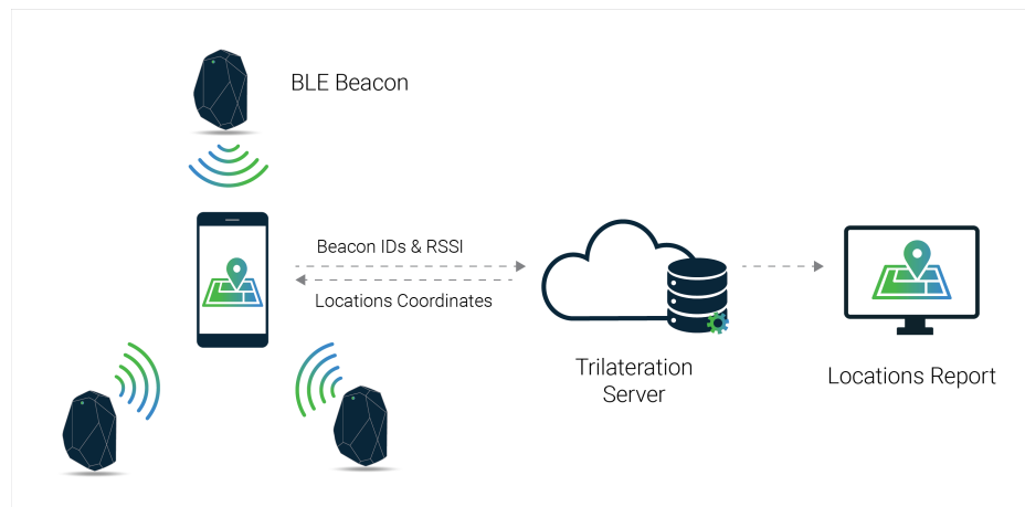
Figure 2.13: BLE indoor tracking through RSSI [5]
