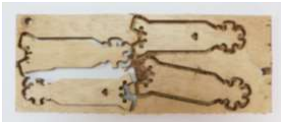
Fig. 1. CNC cut component from plywood
