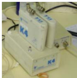
Fig.3 - K4b 2 – Breath by Breath Pulmonary Gas Exchange
