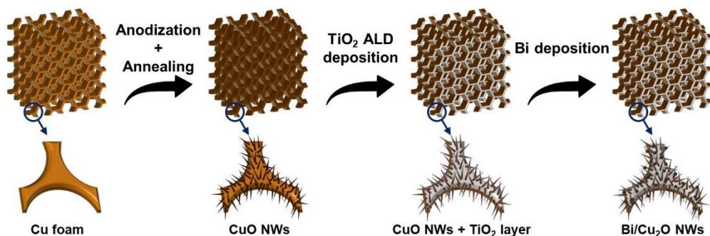
Figure 5.1. Experimental procedure used for the electrocatalysts preparation.
