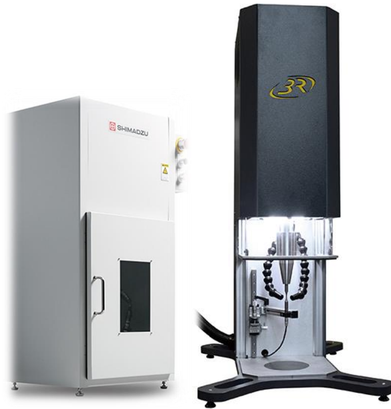
Figure 2.5 - Commercially available UFT machines (left - Shimadzu USF200; right – 3R MEG20) [5] [6]
