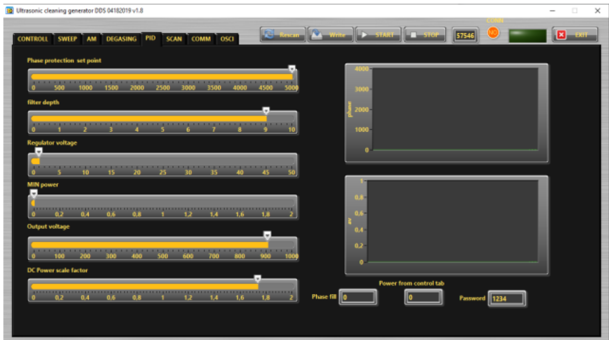
Figure 3.7 - PID tab of the generator software
