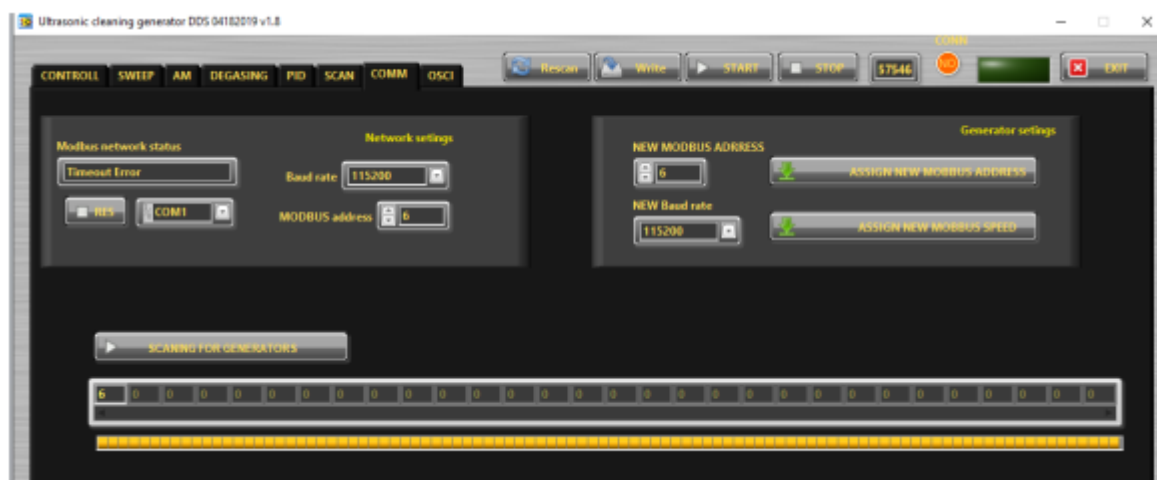
Figure 3.4 - COMM tab of the generator software
