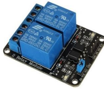
Figure 3.24 - 5 to 24 V DC relay used
