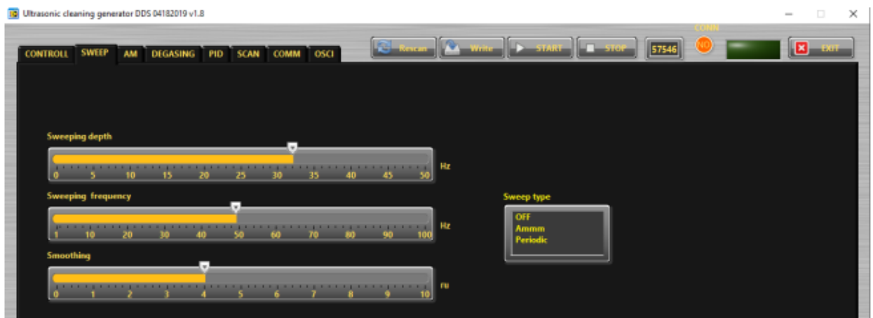
Figure 3.9 - SWEEP tab of the generator software
