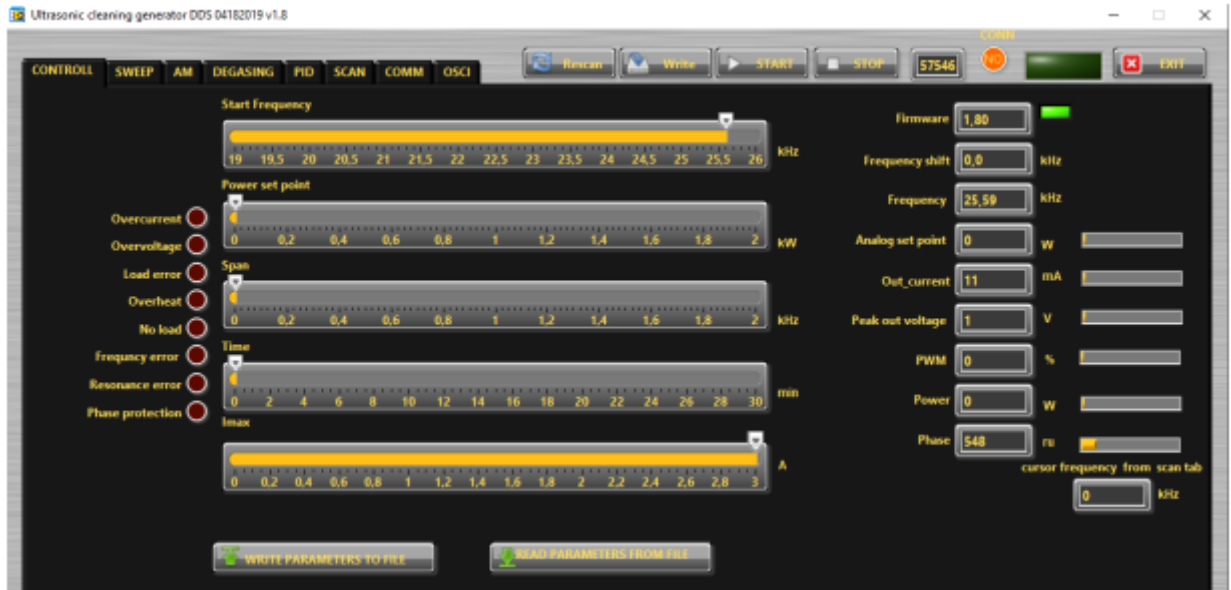
Figure 3.5 - CONTROL tab of the generator software
