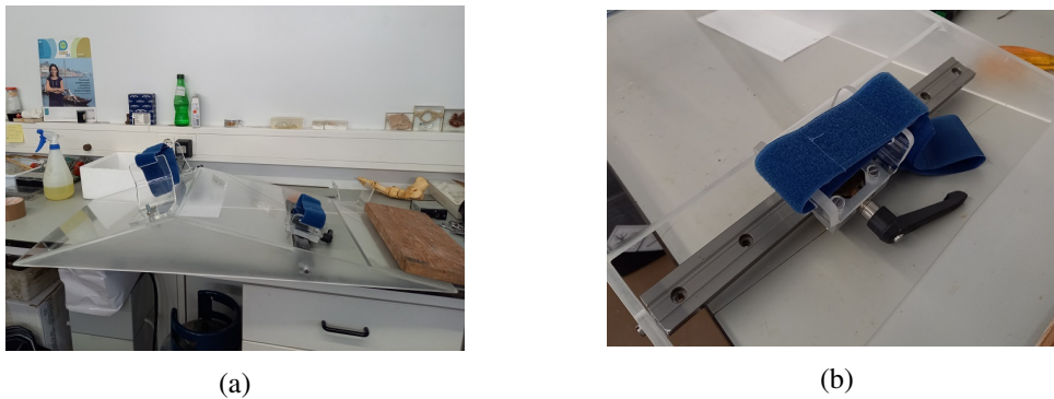
Figure 5.3: Knee positioning system created by the clinical partners of the project: (a) Overall system; (b) Linear guide subsystem.
