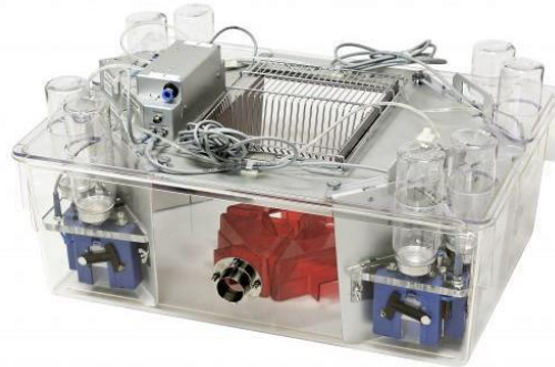
Figure 4.15: Version of the TSE Systems IntelliCage that is used for mice (reproduced from [102])
