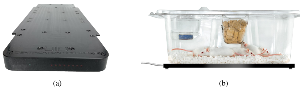
Figure 4.8: (a) Antenna matrix of the UID Mouse Matrix and (b) antenna matrix placed below the cage so that the measurements can be done (reproduced from [90])
