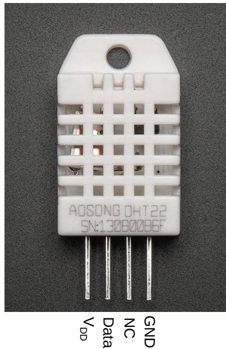
Figure B.4: Pinout of the DHT22
