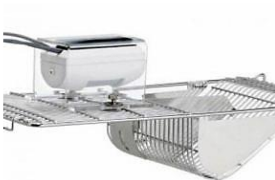
Figure 4.4: Home Cage Infrared Motion Detector attached to the top of a cage (reproduced from [86])
