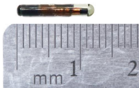
Figure 4.7: Typical appearance of an animal implantable RFID tag (reproduced from [89])
