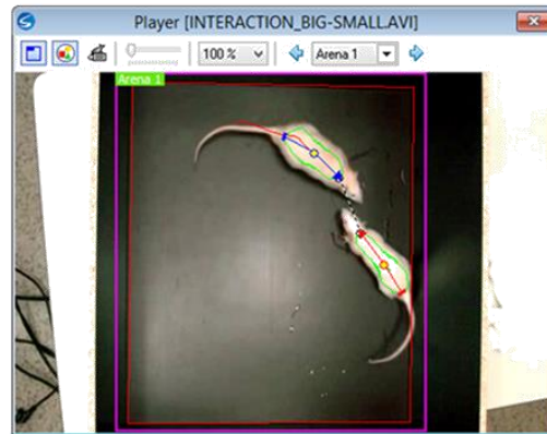
Figure 4.5: Possible interface of the SMART Video Tracking System. The module to detect the head, centre of mass and base of the tail, and the module to track multiple animals are being used. The simultaneous use of both these modules enables the software to better recognize the type of interaction that is happening between the animals (reproduced from [87])
