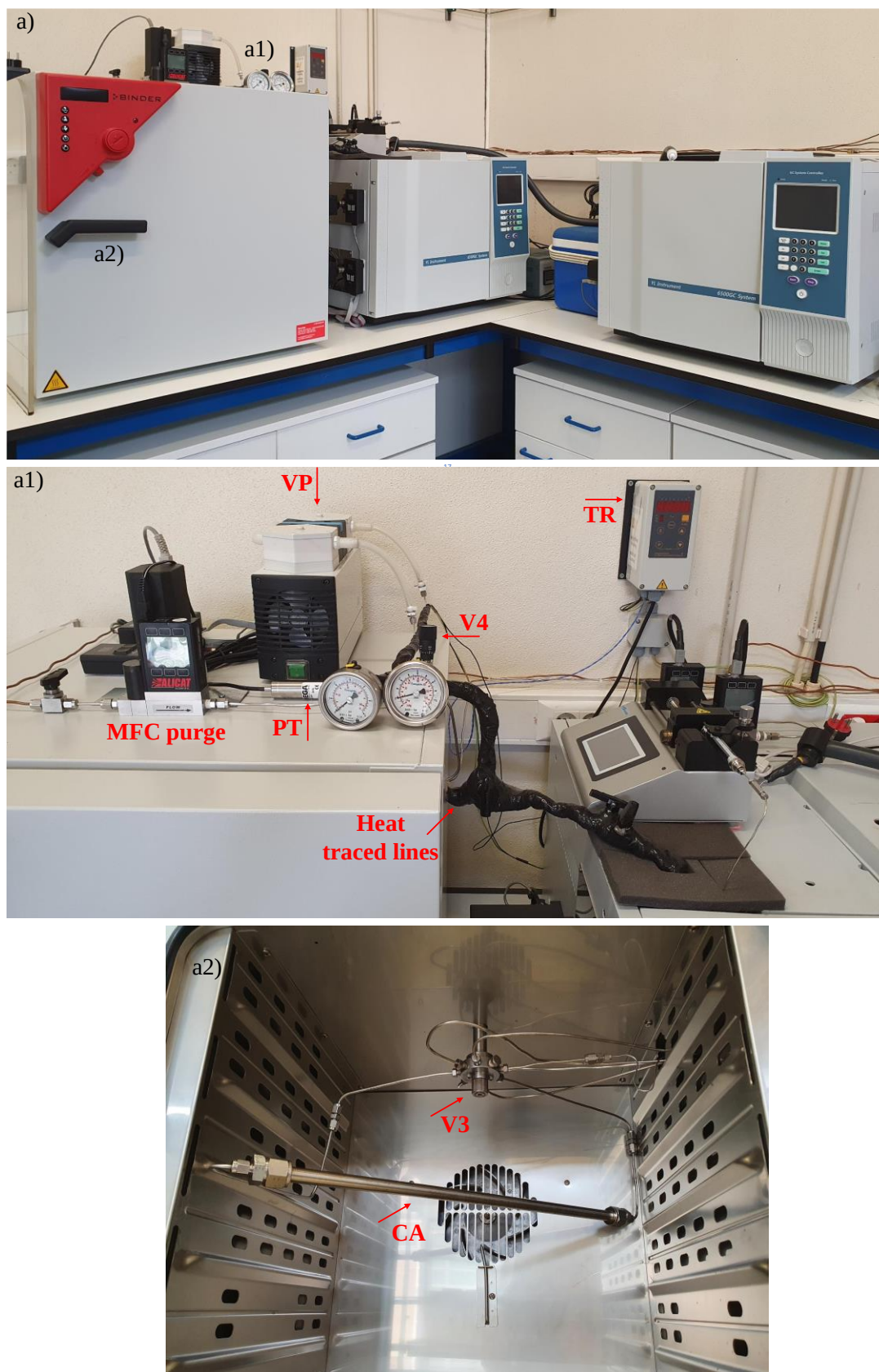
Figure 3.7 | Real view of the screening apparatus upgraded to perform adsorption studies on continuous cyclic operation: a) front view of the complete experimental unit; a1) close-up of the new devices incorporated on the system, showing MFC, PT, VP, valve (V3), TR and heat traced lines, and a2) internal view new HO assembled with a switching valve (V3) and CA.
