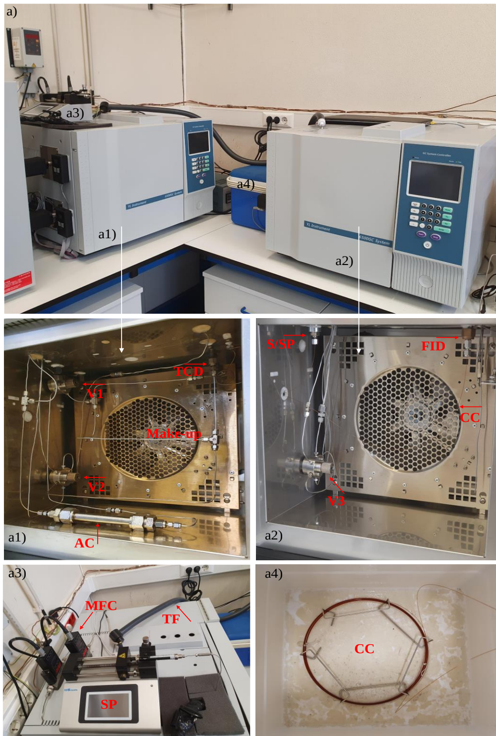
Figure 3.1 | Real view of the screening apparatus developed to measure single and multicomponent breakthrough curves of pentane and hexane isomers: a) front view of the complete experimental unit; a1) internal view of the preparative GC, with visible switching valves (V1) and (V2), AC, streams, and inlet of the TCD; a2) internal view of the analytical GC, with visible sampling valve, the outlet of S/SP injector and inlet of the FID; a3) close-up of the SP and MFC's, and a4) close-up of CC.
