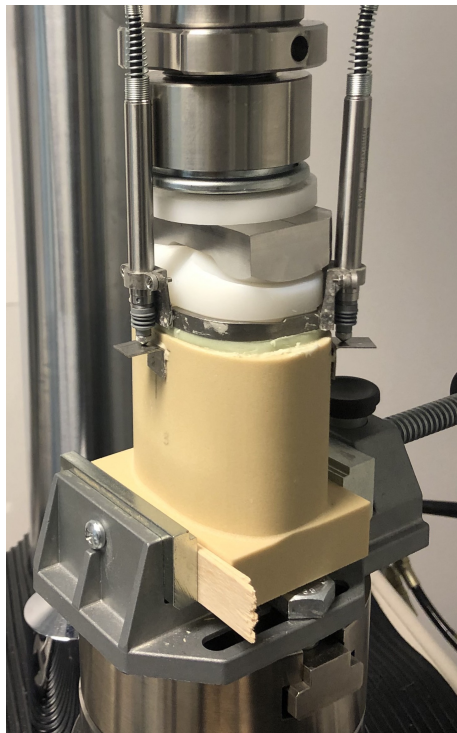
Figure 4.3: Stability test ongoing. The figure shows LVDT's 3 and 4.
