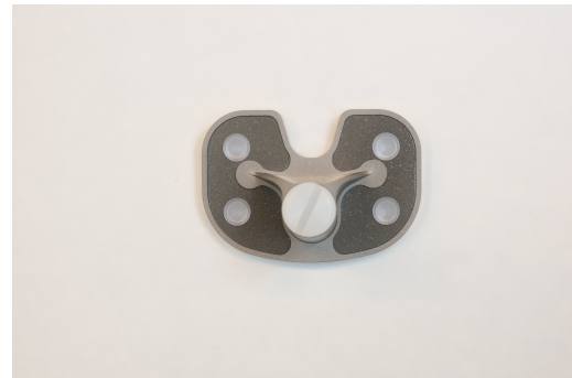
Figure 3.2: Bottom View From a NexGen 3° Stem Tibial Plate (PreCoat) Implant showing the Cement Pockets, the PMMA coating, and design changes.
