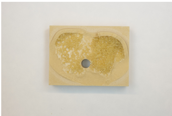
Figure 5.16: Top view from a bone failure (sample n°05).
