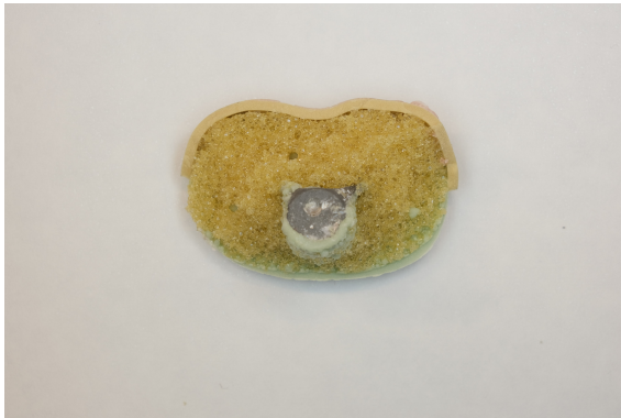
Figure 5.14: Top view from a failure between the bone and the bone-cement with the crack starting at the cement interface and spreading to the bone (sample n°32).
