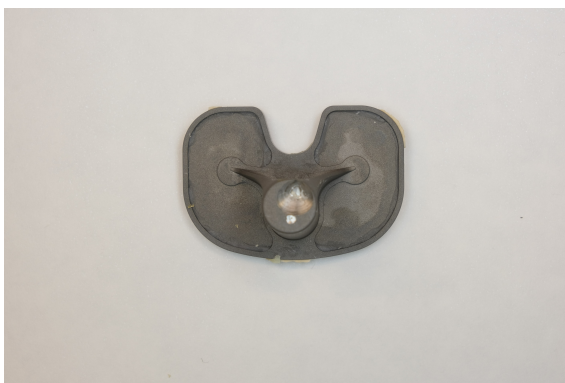
Figure 5.18: Top view from a common implant detachment failure from the implant point of view (sample n°31).
