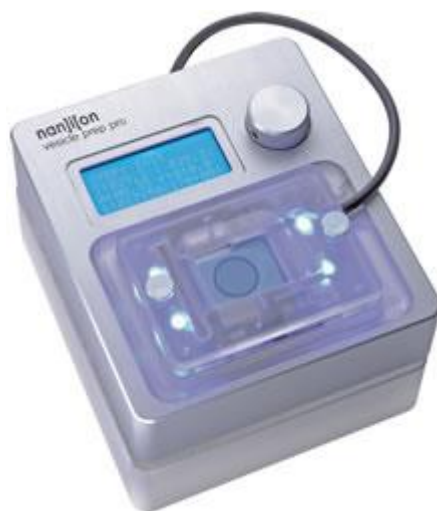
Figure 2. 4 - Vesicle Prep Pro. Equipment produced by Nanion Technologies for electroformation of GUVs.
