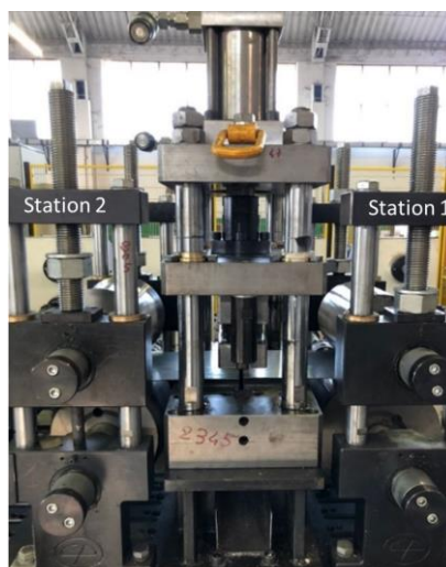
Figure 55 – Cutting operation between stations 1 and 2.
