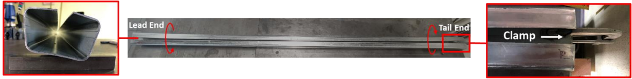
Figure 69 – Fixing the tail end web of the part for twist angle measurement.
