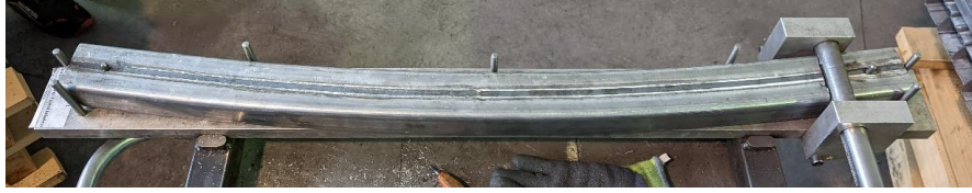
Figure 62 – Stamping and punching control with a calibrator.
