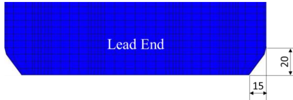
Figure 191 – Chamfer used for the base model.
