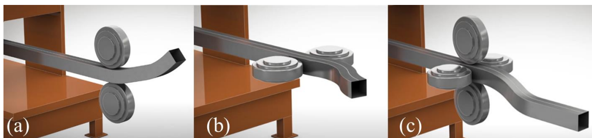
Figure 3 – Examples of bending stations added at the end of the roll forming line: (a) change of shape in one direction; (b) change of shape in two directions;(c) change of shape in three directions. Adapted from(World Auto Steel 2020).
