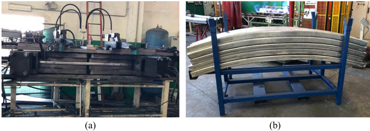
Figure 59 – (a) Stretch bending machine; (b) Stretch bent part.
