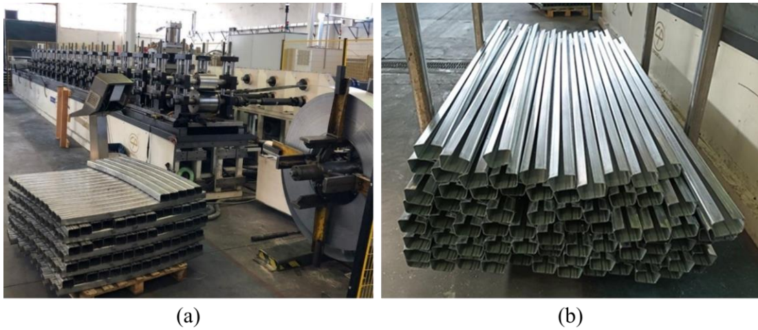
Figure 53 – Roll forming line of Coproget II.
