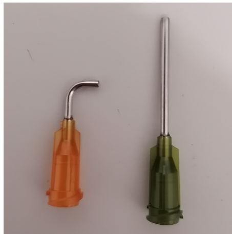
Figure 2.13: Needles used in the set-up for flow analysis using \mu -PIV (left) and for punching (right).
