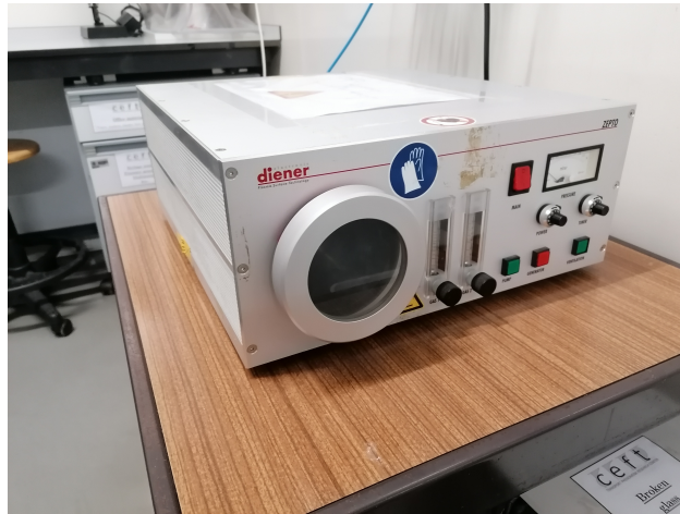
Figure 2.15: Device used for plasma-bonding the PDMS layers and the glass microscopic slides.
