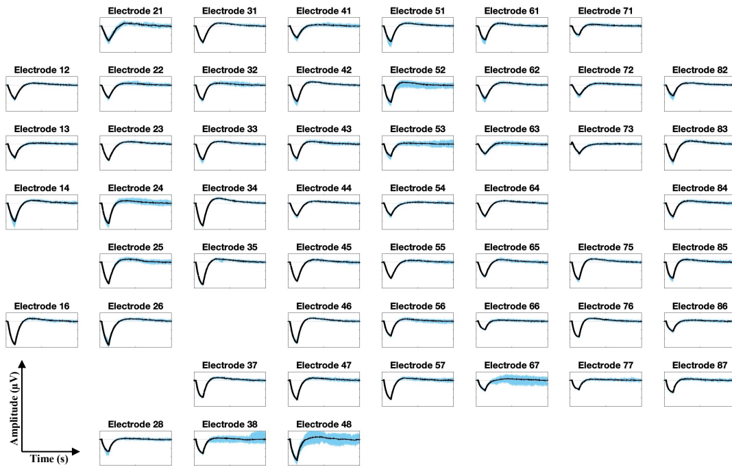
Figure 5.7: Representativeness of the average waveshape of signal's response to stimuli (traced in black), displayed in position of recording, with the maximum deviations (blue areas). Note: subplots are presented with different ranges in y-axis to enhance the visualization of the variation.
