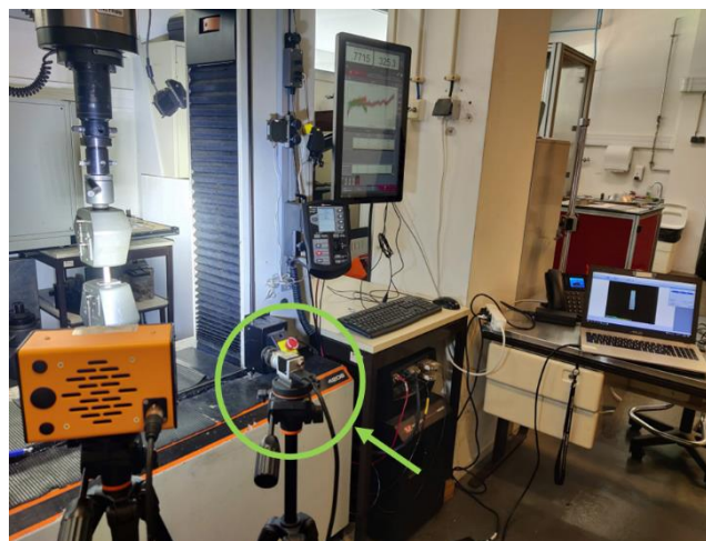
Figure 20 - DIC set-up with tensile test machine. DIC camera is inside the green circle and the orange box is the light source.
