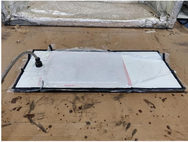
Figure 33 - Vacuum bag before curing
