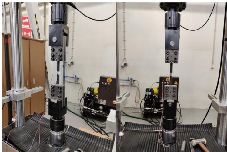
Figure 23 - Stiffness method 1 test set-up
