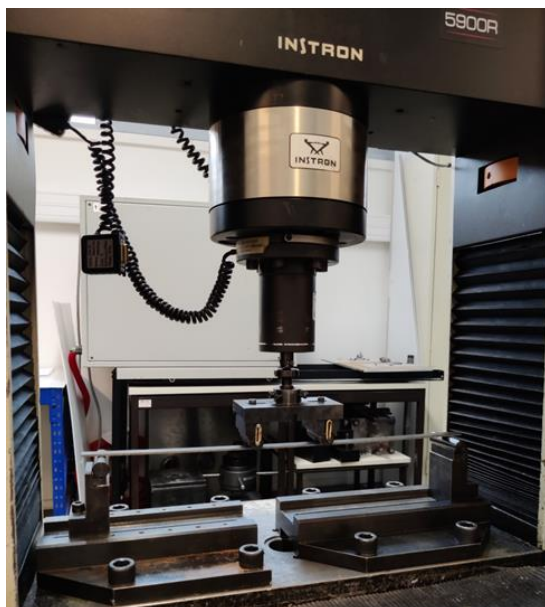
Figure 24 - 4-point flexural test setup
