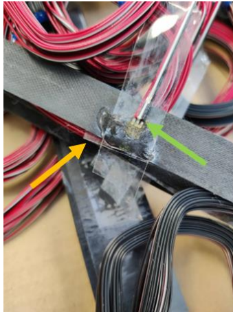
Figure 21 - Strain gauges installed on the 0-degree samples (orange arrow: longitudinal strain gauge; green arrow: transverse strain gauge)
