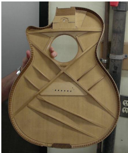
Figure 2 - X-Bracing on a Cutaway Taylor Acoustic Guitar [15]
