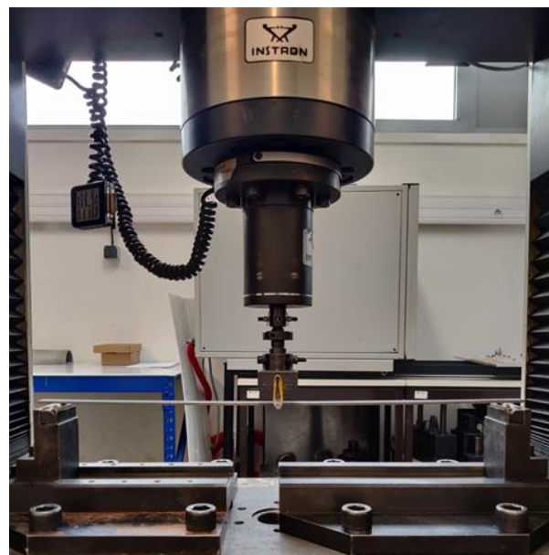
Figure 25 - 3-point flexural test setup
