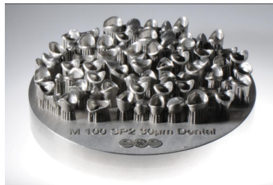
Figure 2.10: Lasersintered CoCr Crowns [36].
