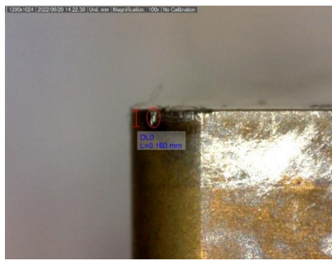
Figure 5.23 - Flank surface of insert "603" exhibiting notching after machining alloy 1 at v_c=150 m/min and a_p=0.15 mm: a) f=0.1 mm/rev after 105 seconds of cutting; b) f=0.2 mm/rev after 65 seconds of cutting.
