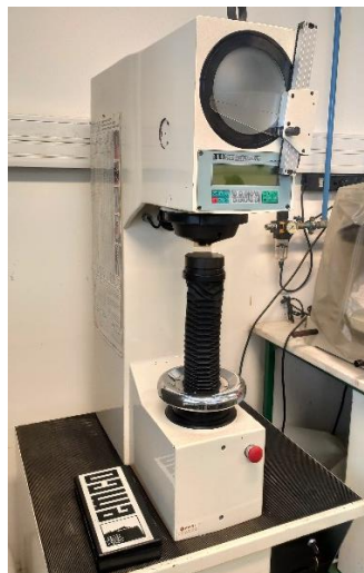
Figure 4.3 - EMCO Test M4U-075 hardness measurement machine.
