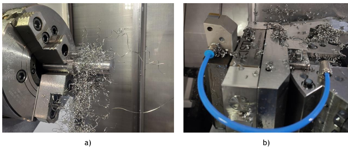
Figure 5.38 - Chip formation: a) chips tangled around the workpiece; b) discontinuous chips.
