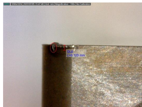
Figure 5.23 - Flank surface of insert "603" exhibiting notching after machining alloy 1 at v_c=150 m/min and a_p=0.15 mm: a) f=0.1 mm/rev after 105 seconds of cutting; b) f=0.2 mm/rev after 65 seconds of cutting.
