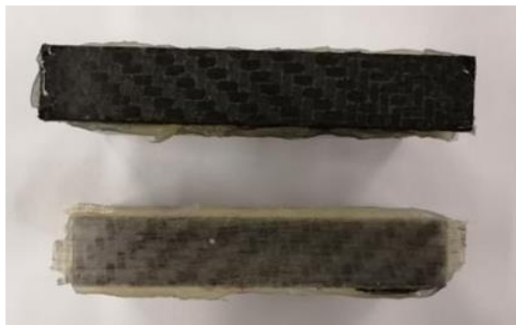
Figure 112 - CT specimen 5 after failure.
