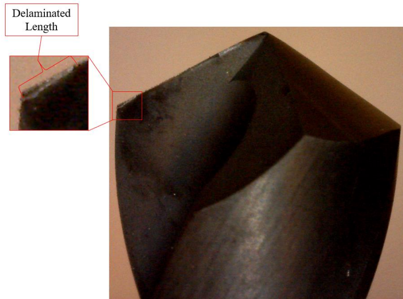
Figure 89 - Rake face of drilling tool after 950 drilled holes, with highlight on coating delamination.
