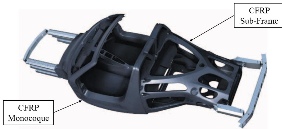
Figure 1 - Porsche Carrera GT chassis, sub-frame and crash structures (adapted from [8]).
