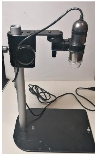
Figure 51 - DinoLite AM-4013MZTL digital USB microscope.
