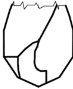
Figure 18 - Double-point angle twist drill (adapted from [25]).
