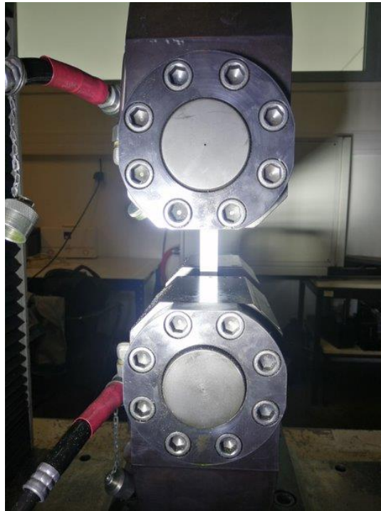
Figure 28 - Tensile testing setup with hydraulic grips.
