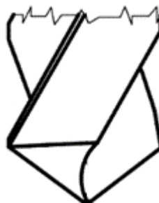
Figure 17 - Conventional twist drill (adapted from [25]).
