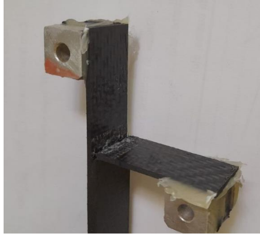
Figure 111 - DCB specimen 5 fractured after being removed from the testing machine.
