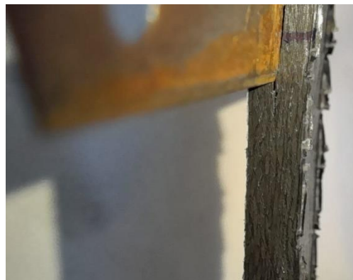
Figure 103 - Usage of a razor blade to facilitate crack propagation before testing DCB specimen 4.
