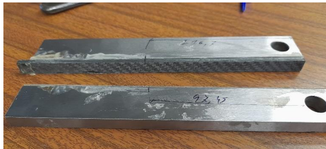
Figure 114 - Final DCB specimen after failure.
