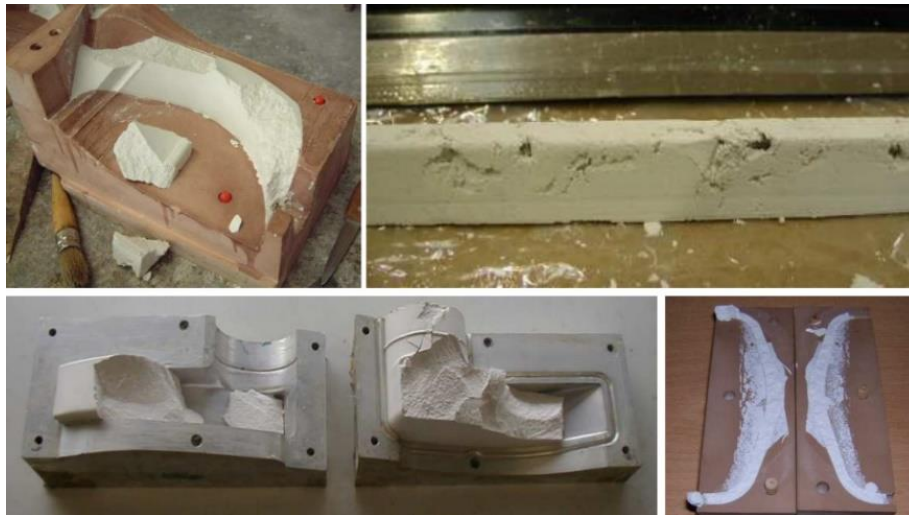
Figure 59 - Aquapour™ production common problems, adapted from [105].
