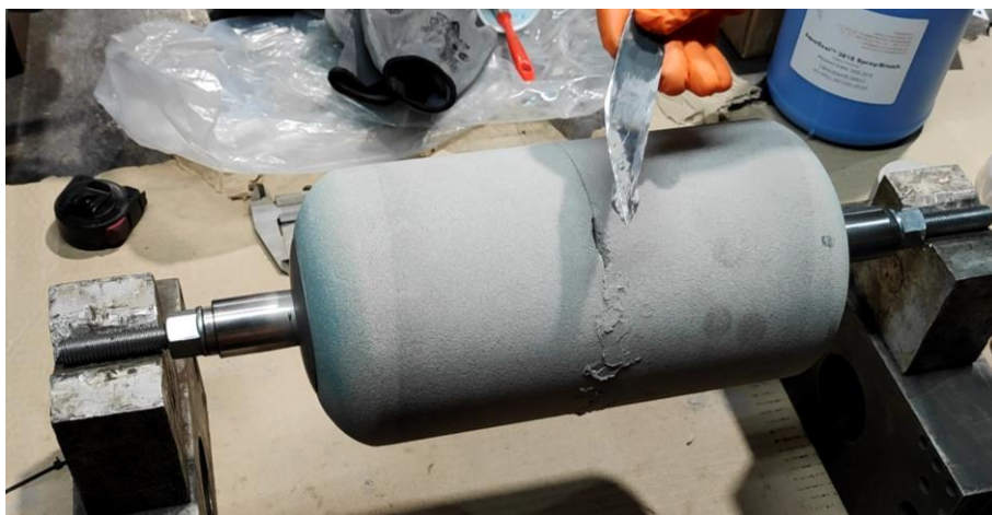
Figure 73 - Photo of the application of Aquafill™ to patch the gap between the two cylindrical blocks.
