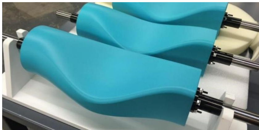
Figure 28 - Example of ExOne 3D printed mandrels with coating [68].
