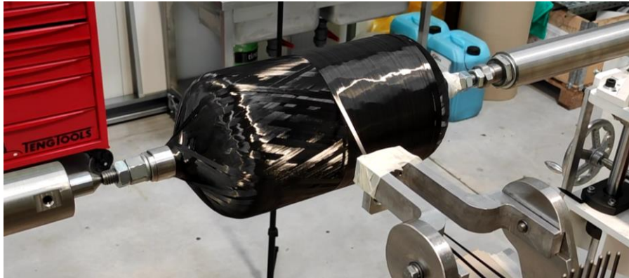
Figure 82 - Hoop layer overwrap with dry fibers.
