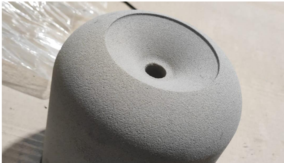
Figure 88 - Photo of the machined dome and polar boss seating surface.
