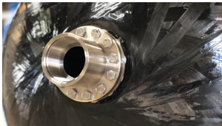
Figure 41 - Polar boss interface in an Infinite Composites pressure vessel, adapted from [102].
