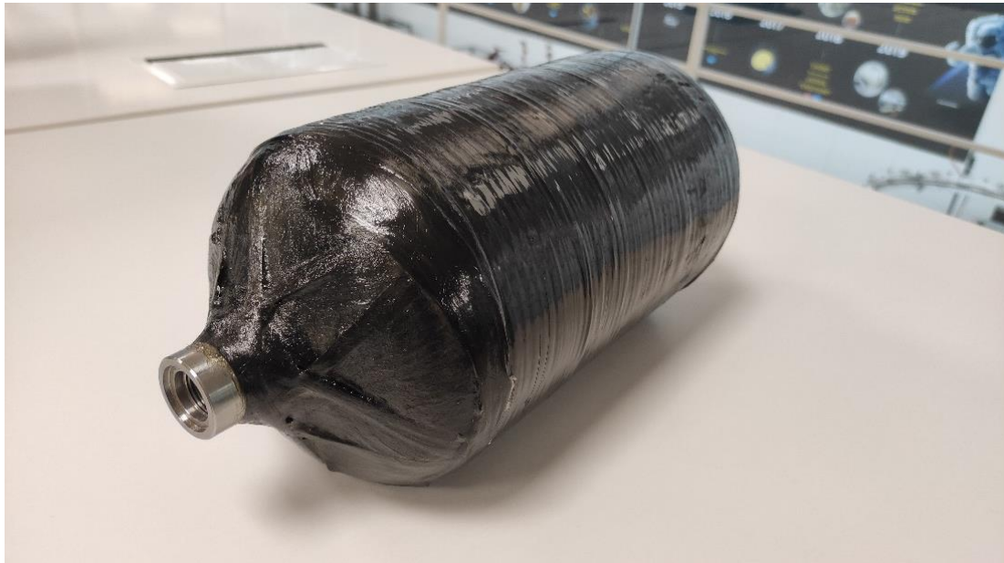
Figure 91 - First linerless COPV prototype produced in the FHP company.
