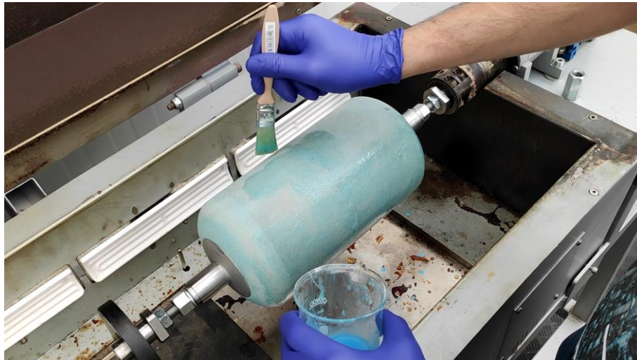
Figure 74 - Application of the Aquaseal™ paint in the mandrel fixed to the cure oven.
