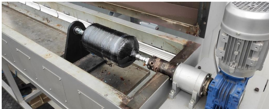
Figure 86 - Pressure vessel at the curing stage in the oven.
