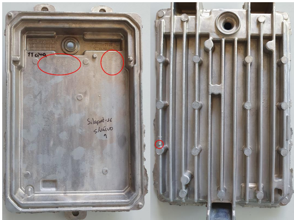
Figure 88: Blistering on conventionally injected part no.1.
