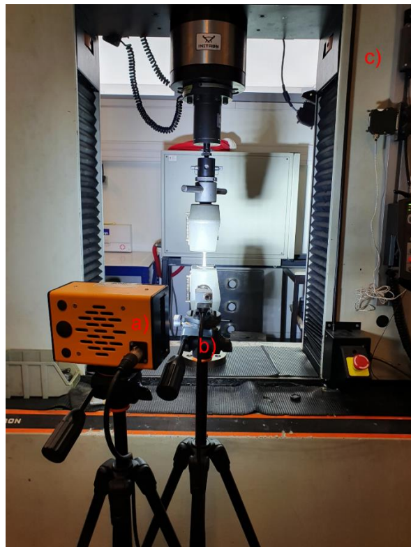
Figure 48: a) spotlight; b) data acquisition camera; c) Instron 5900R machine.
