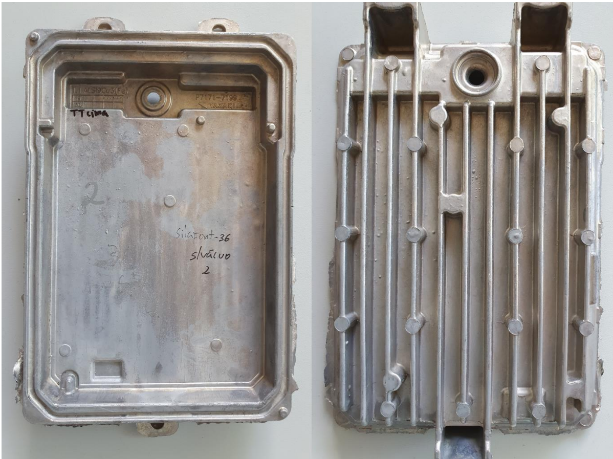
Figure 139: Blistering on conventionally injected part no.2.
