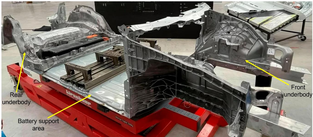
Figure 36: Model Y chassis. Adapted from [58].
