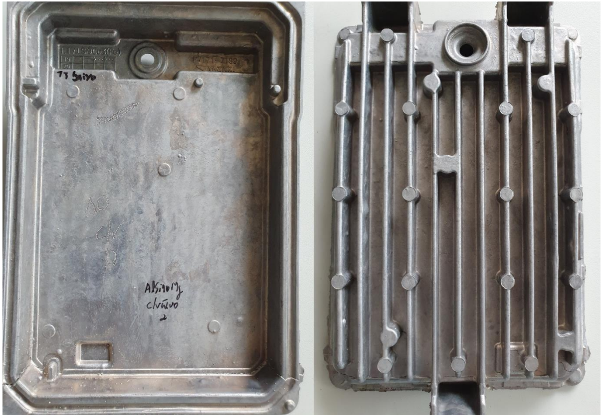
Figure 133: Blistering on vacuum injected part no.2.
