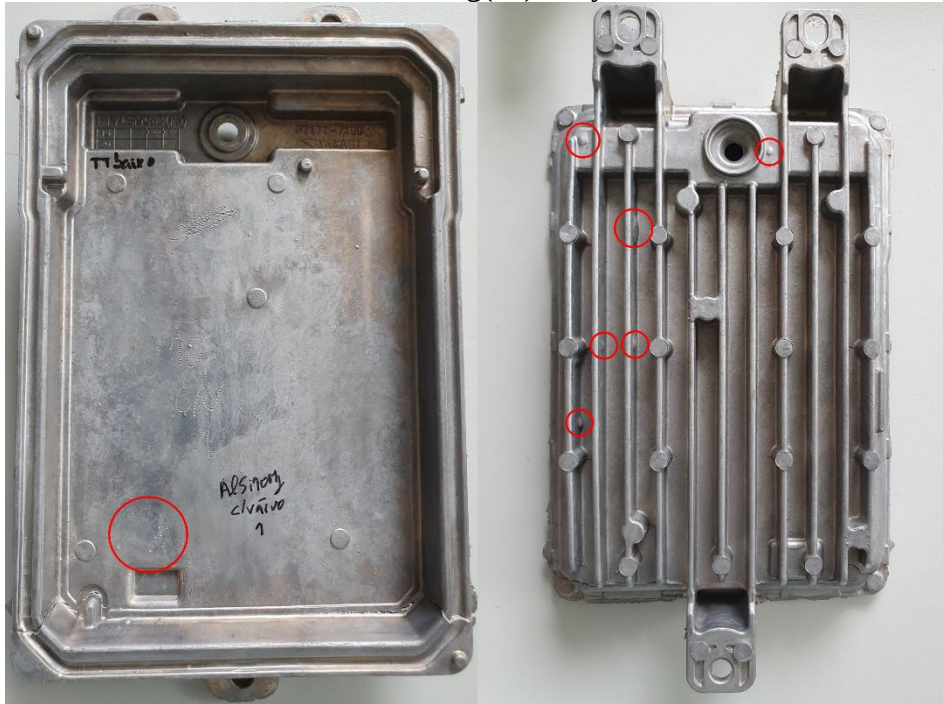
Figure 85: Blistering on vacuum injected part no.1.
