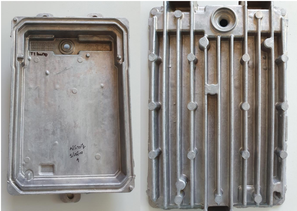
Figure 135: Blistering on conventionally injected part no.1.
