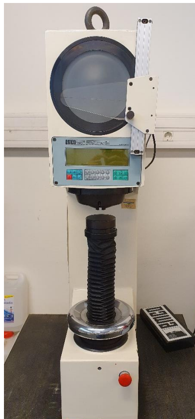
Figure 51: EMCO M4U-075 hardness tester.
