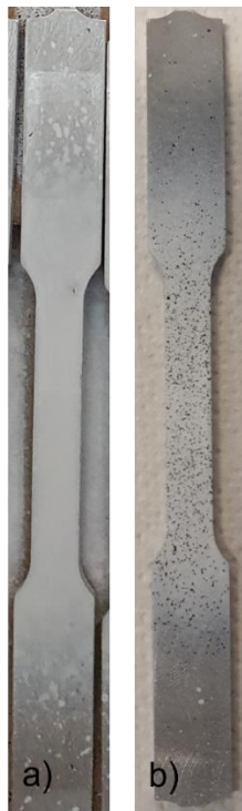
Figure 47: a) specimen painted with a white layer; b) specimen with black dots on the white layer.
