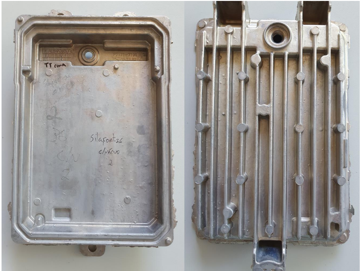
Figure 137: Blistering on vacuum injected part no.2.
