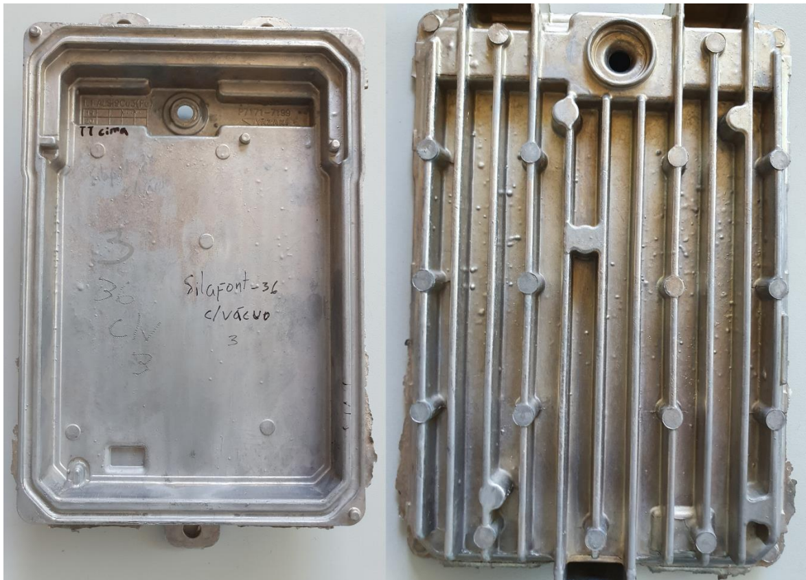
Figure 138: Blistering on vacuum injected part no.3.
