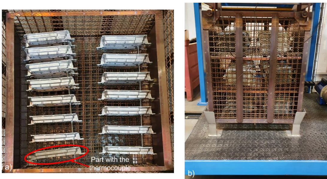
Figure 54: a) Parts placed in the basket; b) Parts before heat treatment.
