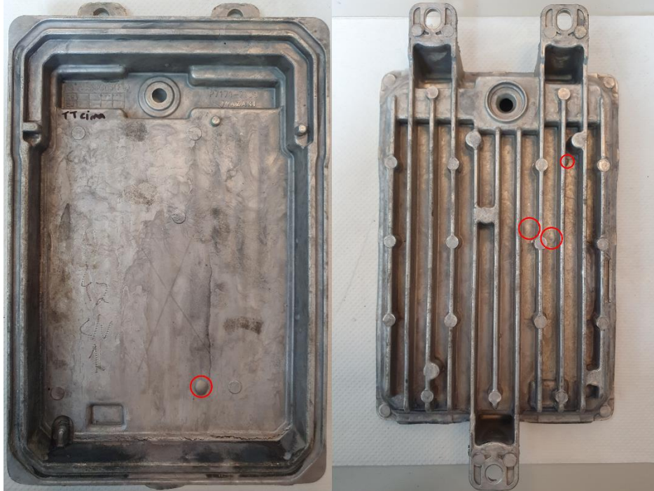
Figure 91: Blistering on vacuum injected part no.1.
