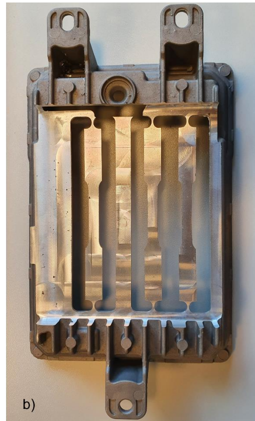
Figure 41: a) CAD model of the specimen positioning - bottom view of the part; b) Positioning the specimens after machining - top view of the part.
