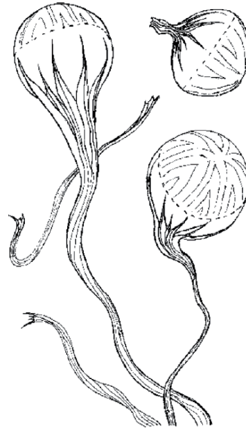
Figure 29: Bubbles and their oxide tails [32].
