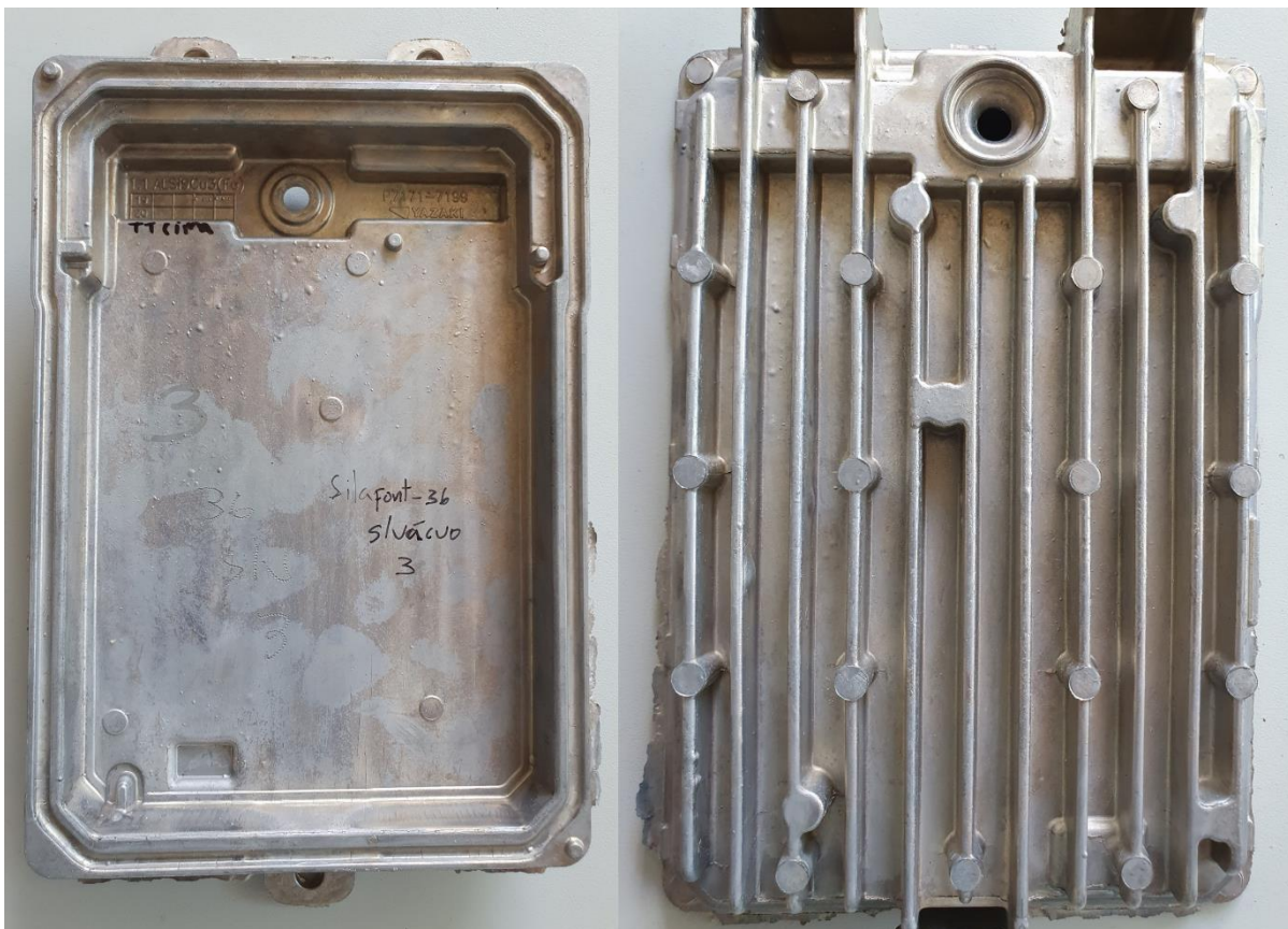
Figure 140: Blistering on conventionally injected part no.3.
