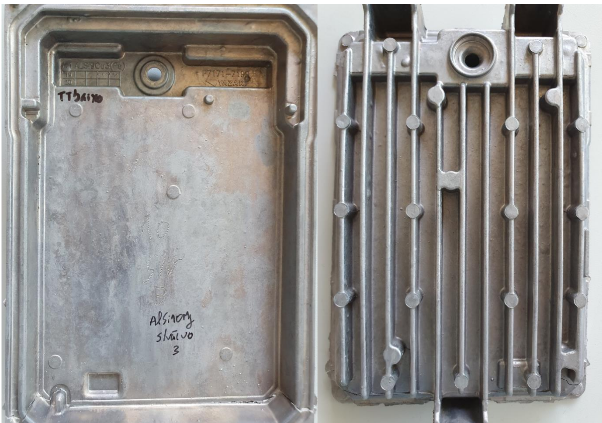
Figure 136: Blistering on conventionally injected part no.3.
