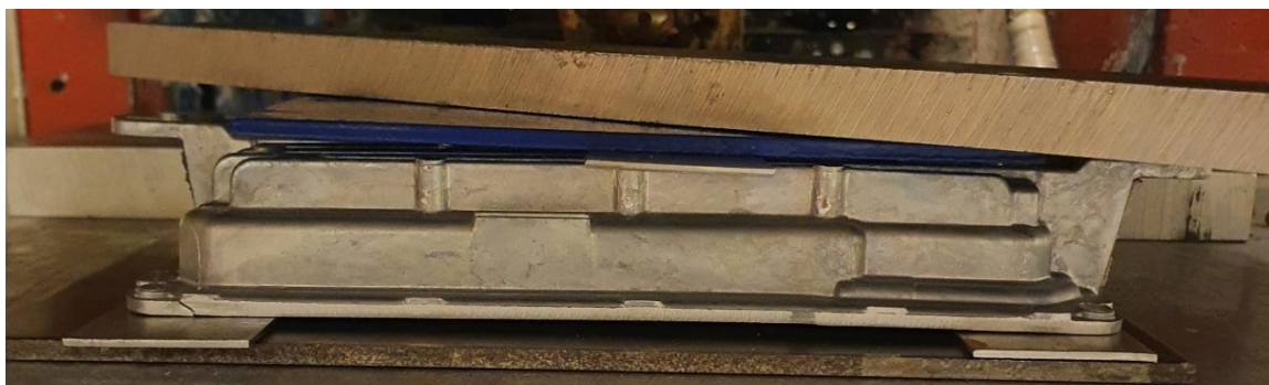
Figure 44: Assembly used to straighten the parts.
