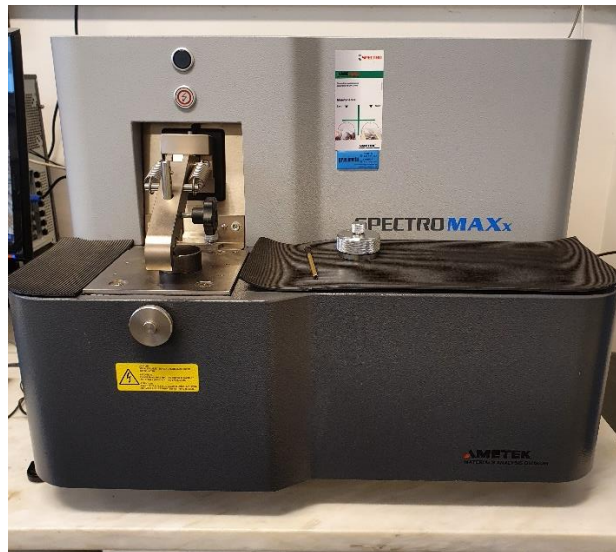
Figure 49: Ametek SPECTROMAXx used in chemical composition analysis.
