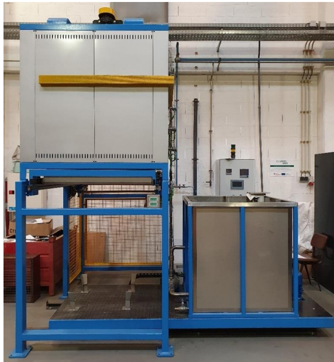
Figure 52: M.J. Amaral forced convection furnace with a chamber of dimensions 600 \times 600 \times 700 \text{ mm}^3 .
