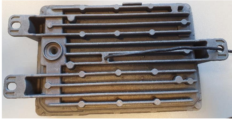
Figure 53: Thermocouple placed on test part.
