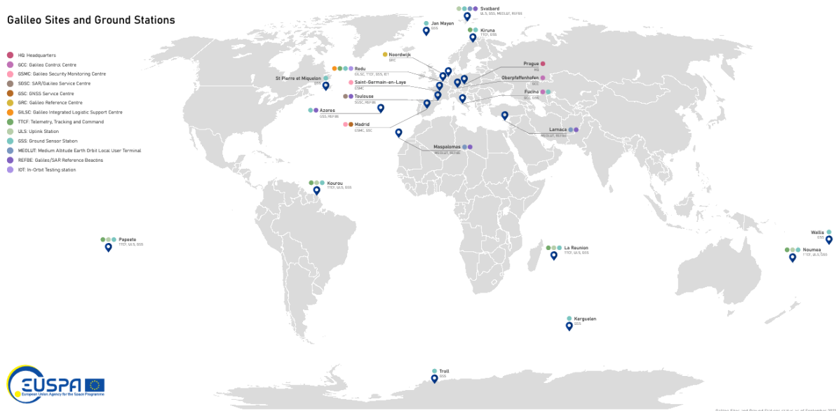
Figura 3.16 – Rede do segmento terrestre do Galileo (European GNSS Service Center, 2021)
