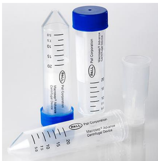
Figure A4. 1K Omega Macrosep Advance Centrifugal Devices (Pall Corporation), used to concentrate protein and dilute salts.
