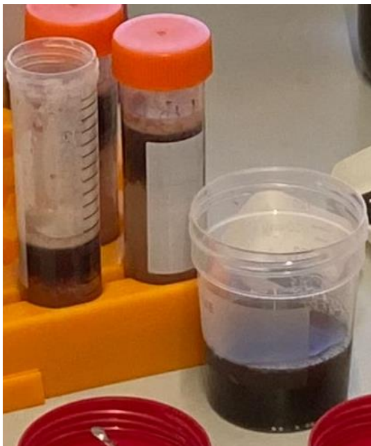
Figure A4. 50 mL falcon tube for centrifuging the acid extract (left) and goblet for the alkaline mixing phase (right).
