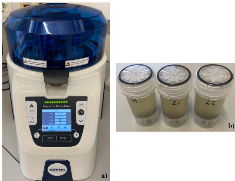
Figure A1. a) Precellys Evolution System; b) 15 mL flasks containing the algal sample, solvent, and ceramic beads.
