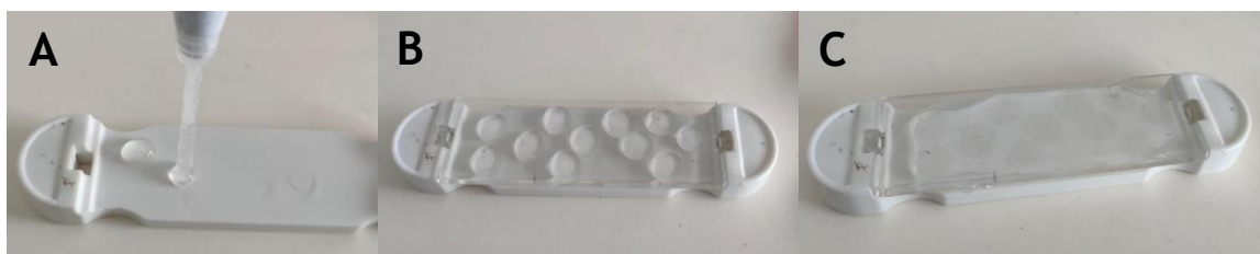
Figure 4.11 – Production of cylindrical pectin hydrogels using QGel® 3D disc caster. A) Deposition of pre-crosslinked hydrogel; B) Internally cross-linked produced hydrogels; C) \text{CaCl}_2 bath (external gelation) for hydrogel reinforcement.
