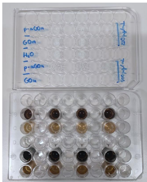
Figure 4.10 – Disposition of GBM dispersions and water control in 48 well-plate to be NIR irradiated. From top to bottom: p-rGOn and GOn at a concentration of 250 µg/mL, water, p-rGOn and GOn at a concentration of 500 µg/mL.
