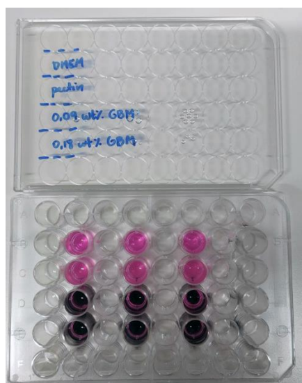
Figure 4.16 – Disposition of produced hydrogels and DMEM control in 48 well-plate to be NIR irradiated. From top to bottom: DMEM; pectin hydrogel (0 wt.% GBM); 0.09 wt.% GBM hydrogel and 0.18 wt.% GBM hydrogel.
