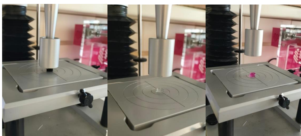
Figure 4.12 – Compression test using the texture analyzer for A) GBM hydrogel; B) pectin hydrogel; C) pectin incubated in DMEM hydrogel samples.
