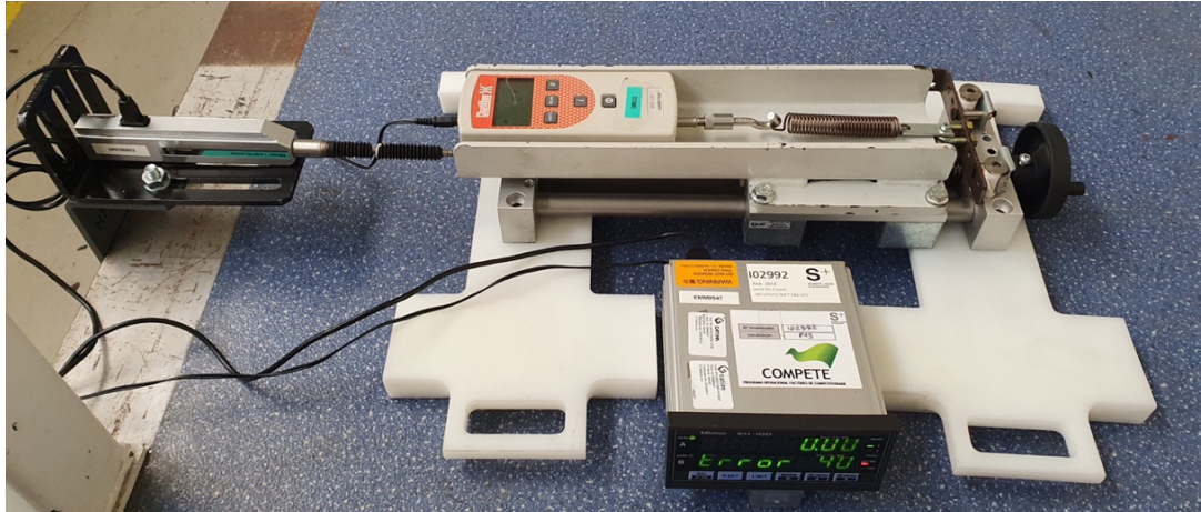
Figure 3.10 - Axial traction test installation with all the measurement devices and test sample in place.
