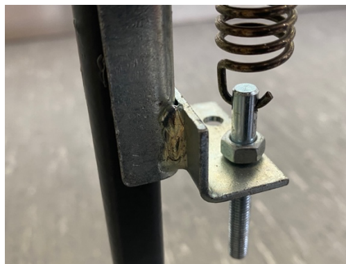
Figure 3.12 - Spring pre-charge adjustment.
