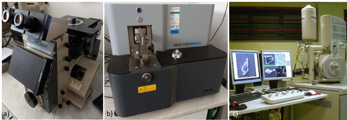
Figure 35 - a) Optical microscope OLYMPUS PMG3; b) spark emission spectroscopy SPECTROMAXx; c) Scanning Electron Microscope (FEI Quanta 400FEG ESEM / EDAX Genesis X4M) at CEMUP
